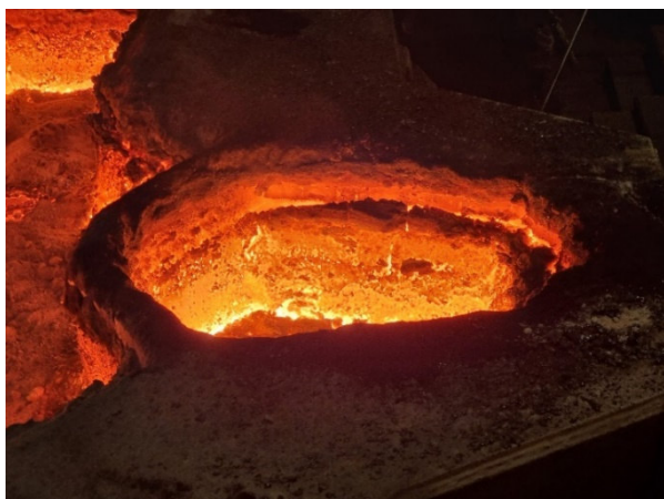
Fig. 6 State of the inlet after the end of the test, after the 16 th melting
