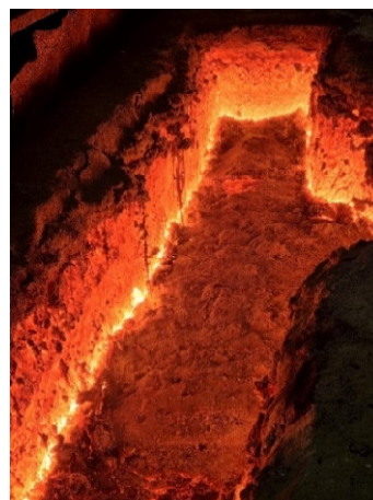
Fig. 7 State of the intermediate pan after the end of the test, after the 16 th melting.
