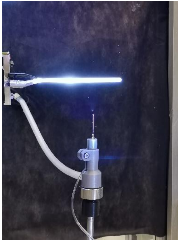
Figure 2 Stable fibre formation using the DC electrospinning method
