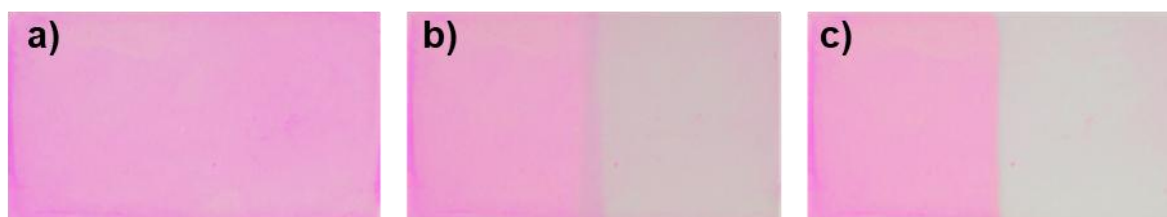
Figure 2 White cement block with TEX45 photocatalyst and RhB at a) 0, b) 4, and c) 26 hours of irradiation
