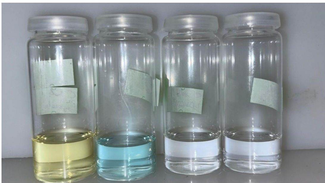
Figure 4 The optical images of the diffusion process of polysulfides of PE separator
