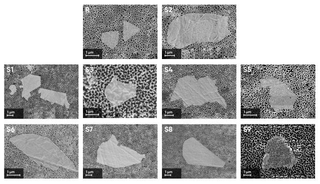
Figure 1 SEM micrographs of synthesised Ti<sub>3</sub>C<sub>2</sub>T<sub>x</sub> nanosheets
