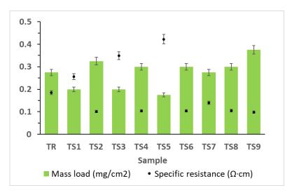
Figure 5 Specific electrical resistance of functionalised cotton fabric versus mass load
