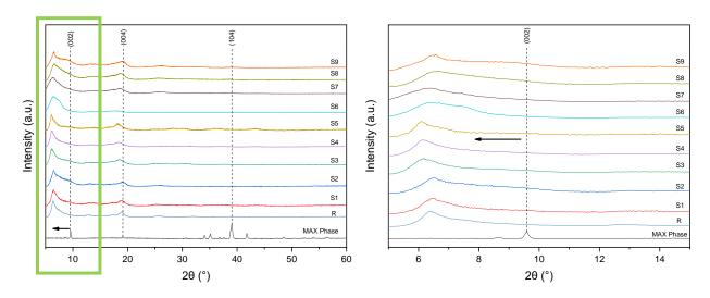
Figure 3 XRD of Ti<sub>3</sub>C<sub>2</sub>T<sub>x</sub>; enlarged detail in the green square on the right
