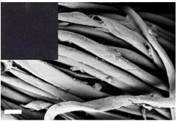
**Figure 4** The selected SEM micrographs of pristine cotton fabric (left); and Ti<sub>3</sub>C<sub>2</sub>T<sub>x</sub>-functionalised fabric, TS2 (right); the scale bar is 20 μm. In the left corners are photographs of untreated (white) and Ti<sub>3</sub>C<sub>2</sub>T<sub>x</sub>-coated fabrics (black)
