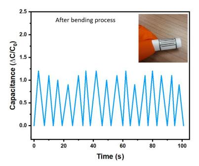
Figure 5 Capacitance change of the sensor after bending-relaxation process.
