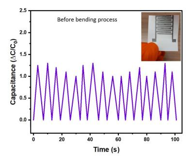
Figure 4 Capacitance change of the sensor before bending process
