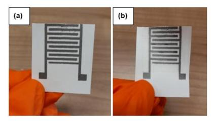
Figure 1 (a) Printed pressure sensor without coating, (b) Printed pressure sensor coated with welding tape
