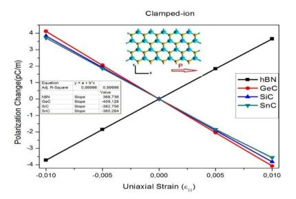
**Figure 2** Applying an uniaxial in-plane strain to SiC induces a change in the polarization perpendicular to the sheet. At low strains, this relationship is linear where the slope gives the e<sub>11</sub> piezoelectric coefficient.
