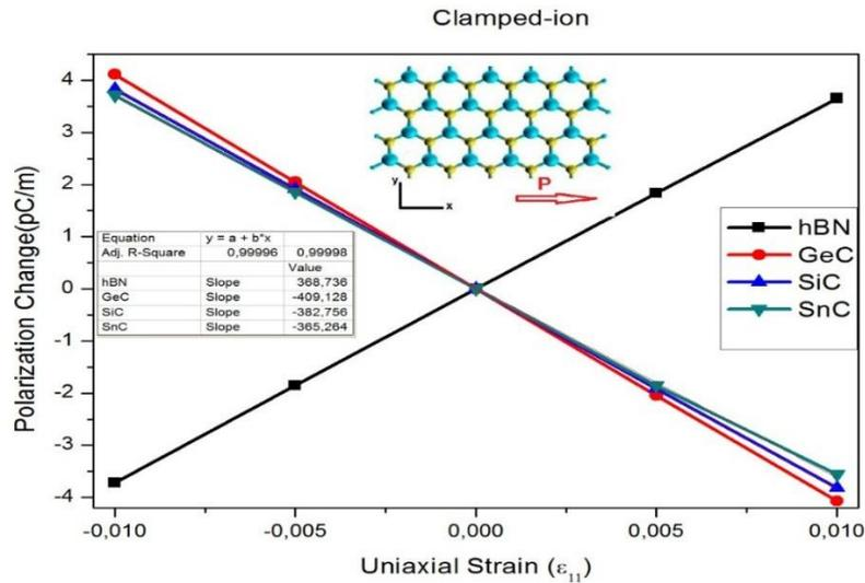
**Figure 2** Applying an uniaxial in-plane strain to SiC induces a change in the polarization perpendicular to the sheet. At low strains, this relationship is linear where the slope gives the  $e_{11}$  piezoelectric coefficient.
