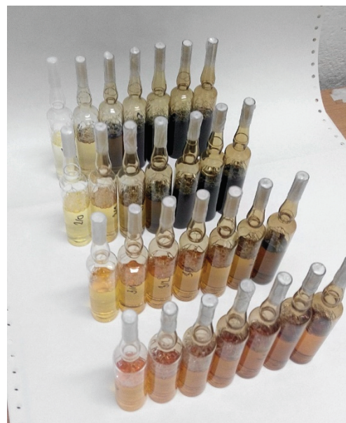
Figure 3 Appearance of irradiated samples. The samples are sorted from the back to the front according to the increasing concentration: 1 mM PtCl 4 , 2 mM, 5 mM and 10 mM and from left to right according to the increasing dose: 0, 4, 8, 12, 16 and 24 kGy
