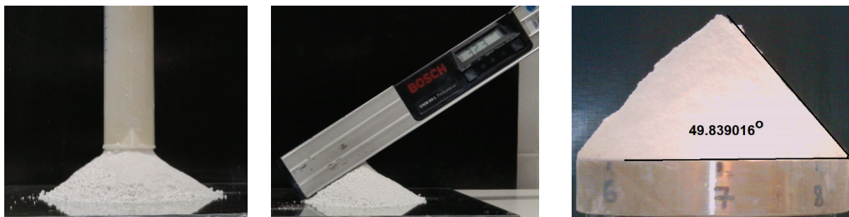
Figure 2 Left - static angle of repose determined by pouring of powder on a horizontal pad for sample A, right - static angle of repose determined by Zenegero method for sample C
