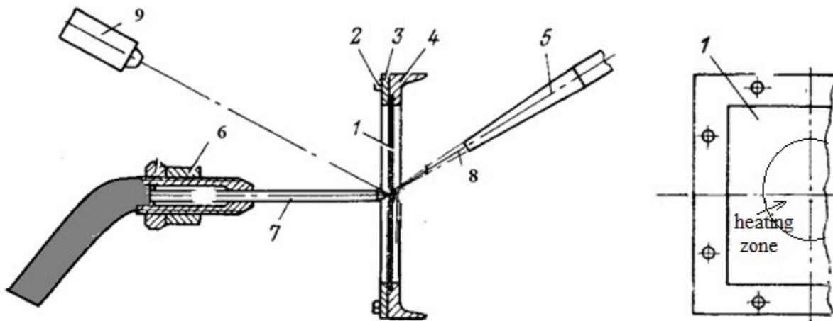
**Figure 1** Scheme fixing for heating and cooling sample: (1) sample; (2) screw for fastening clamp; (3) clamp; (4) frame for mounting the sample; (5) nozzle for the supply of cooling water; (6) acetylene burner; (7) gas-flame jet; (8) water jet; (9) laser pyrometer
