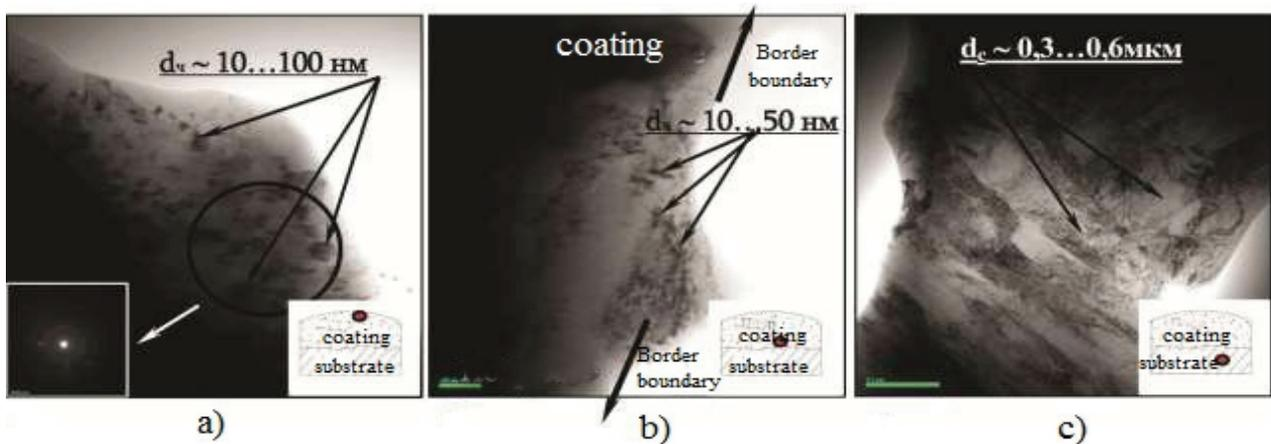
**Figure 4** Fine structure: coatings  $\text{Al}_2\text{O}_3+3\% \text{Ti}$  at a depth of  $\delta \sim 150 \dots 200 \mu\text{m}$  from the interface (a), in the coating-substrate interface (b) and the substrate material (c)
