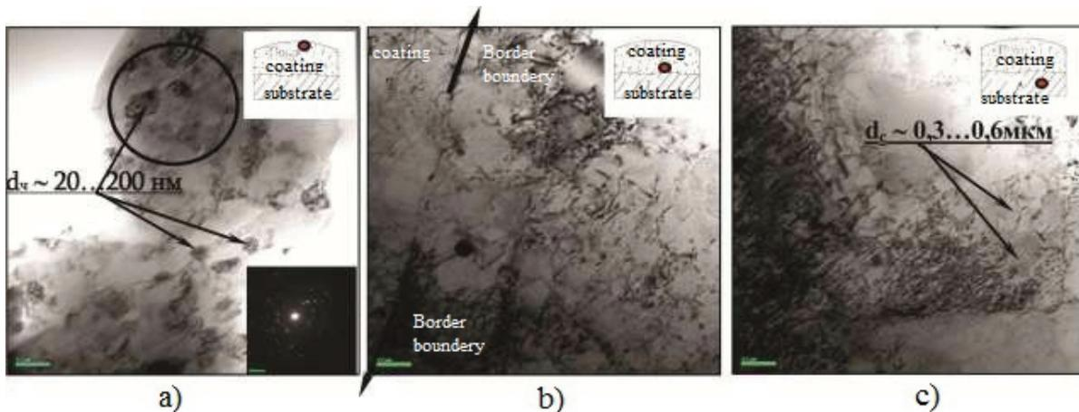
**Figure 5** Fine structure: coatings  $\text{Al}_2\text{O}_3+13\% \text{Ti}$  at a depth of  $\delta \sim 150 \dots 200 \mu\text{m}$  from the interface (a), in the coating-substrate interface (b) and the substrate material (c)
