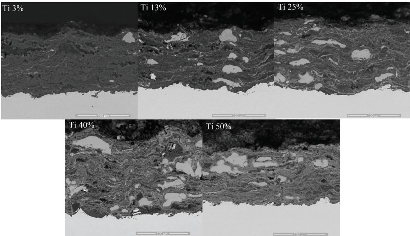
**Figure 2** Structure of the Al<sub>2</sub>O<sub>3</sub>/xTi composite coatings before annealing
