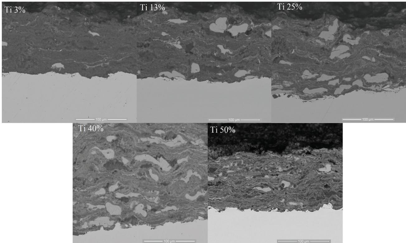
**Figure 3** Structure of the  $\text{Al}_2\text{O}_3/\text{xTi}$  composite coatings after annealing
