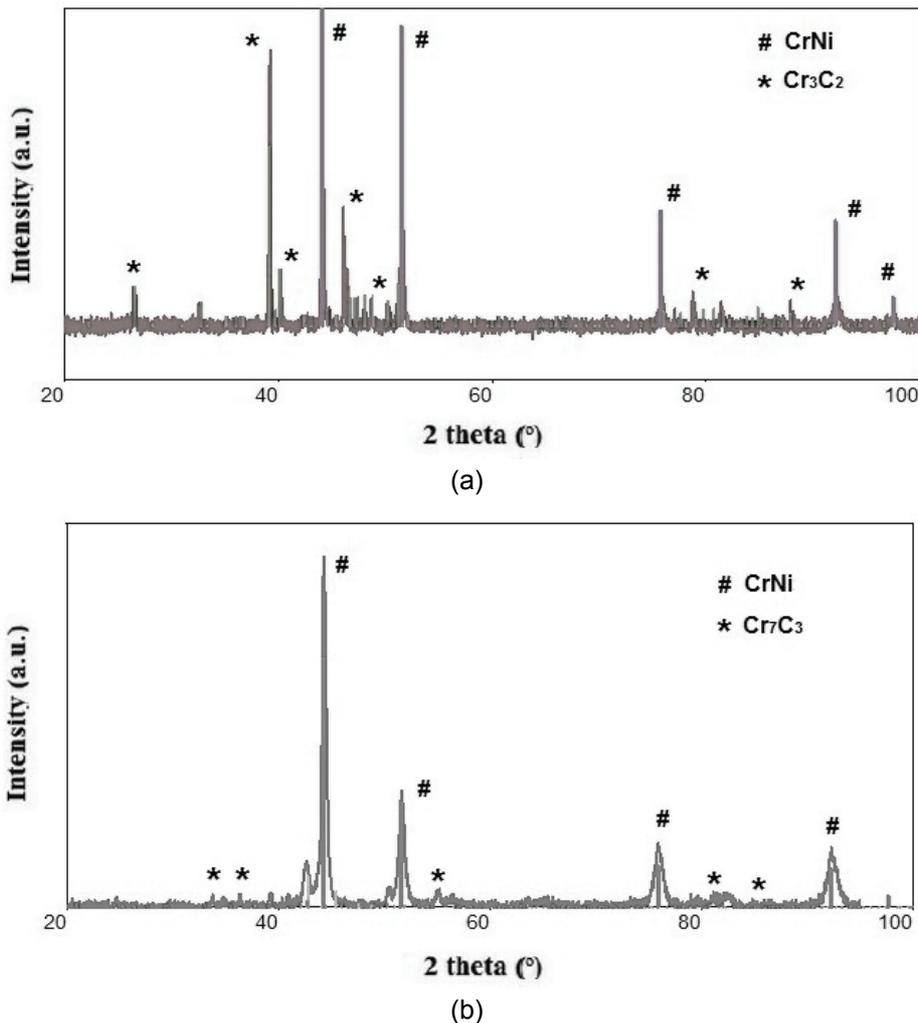
**Figure 3** XRD patterns of the (a) Cr<sub>3</sub>C<sub>2</sub>-25NiCr powder, and (b) the Cr<sub>3</sub>C<sub>2</sub>-25NiCr coating
