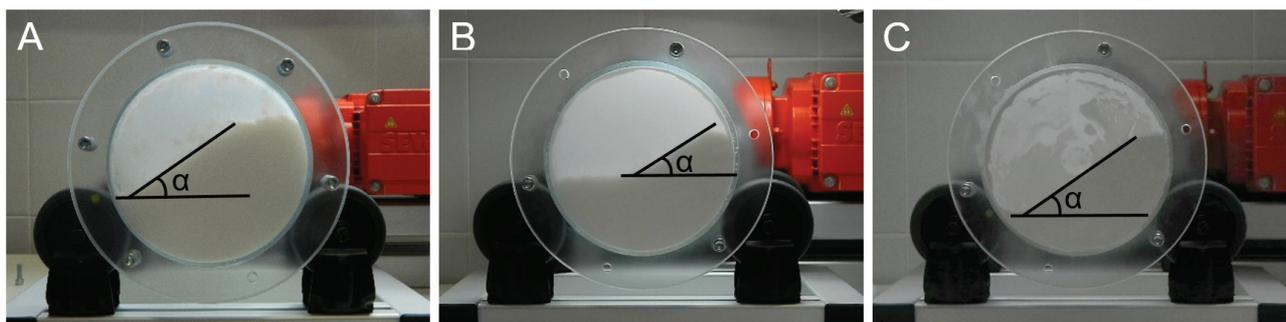
**Figure 5** Angle of repose for Aerosil® 380 (A), Cab-O-Sil® (B) and magnesium stearate (C), 20 rpm
