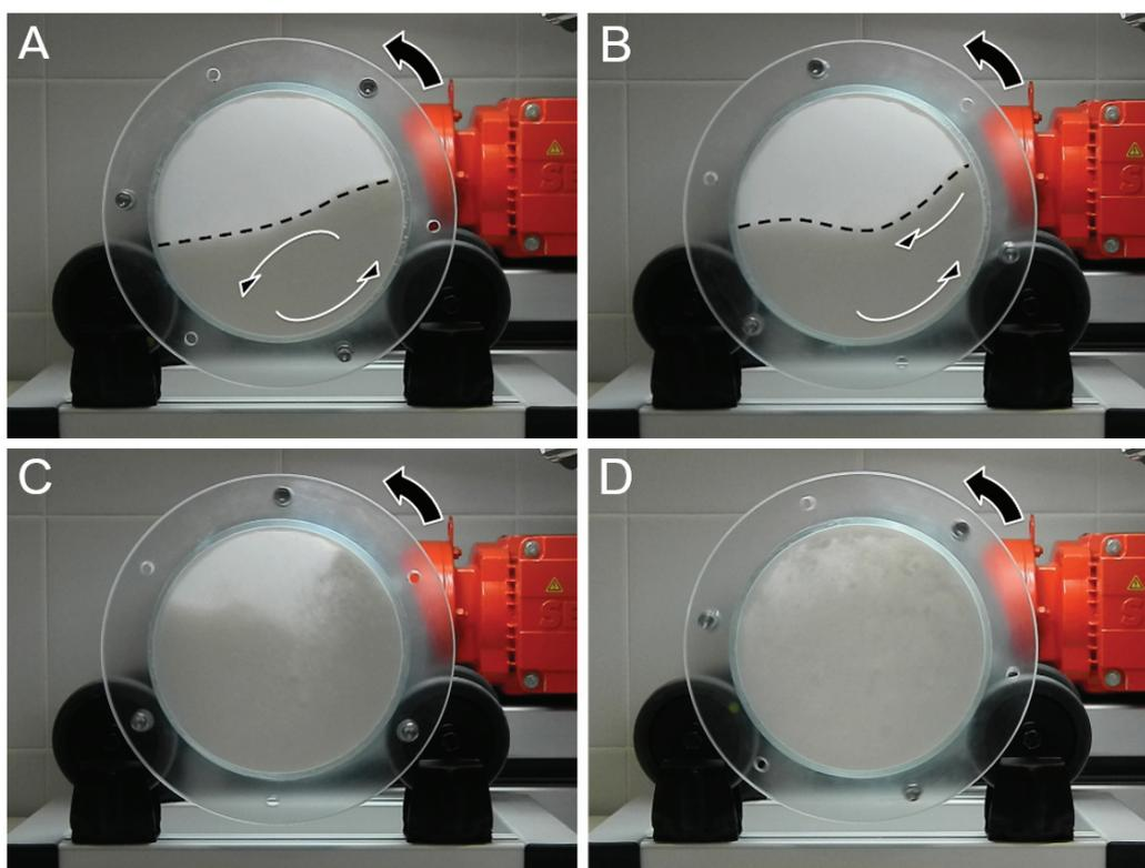
**Figure 3** Dynamic behaviors of Cab-O-Sil<sup>®</sup> with increasing rotating frequency. A - rolling region, B - cascading region, C - swirled, D - dynamic swirled
