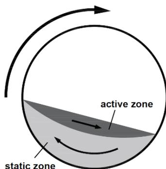
**Figure 4** Active and static zone for magnesium stearate (scheme)
