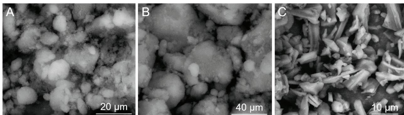
**Figure 1** SEM images of Aerosil<sup>®</sup> 380 (A), Cab-O-Sil<sup>®</sup> (B) and magnesium stearate (C)
