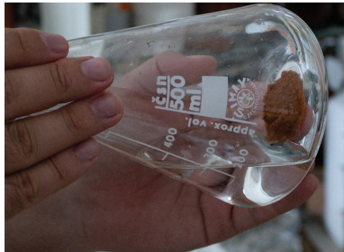
Figure 4 Separation of the biocatalyst with neodymium magnet
