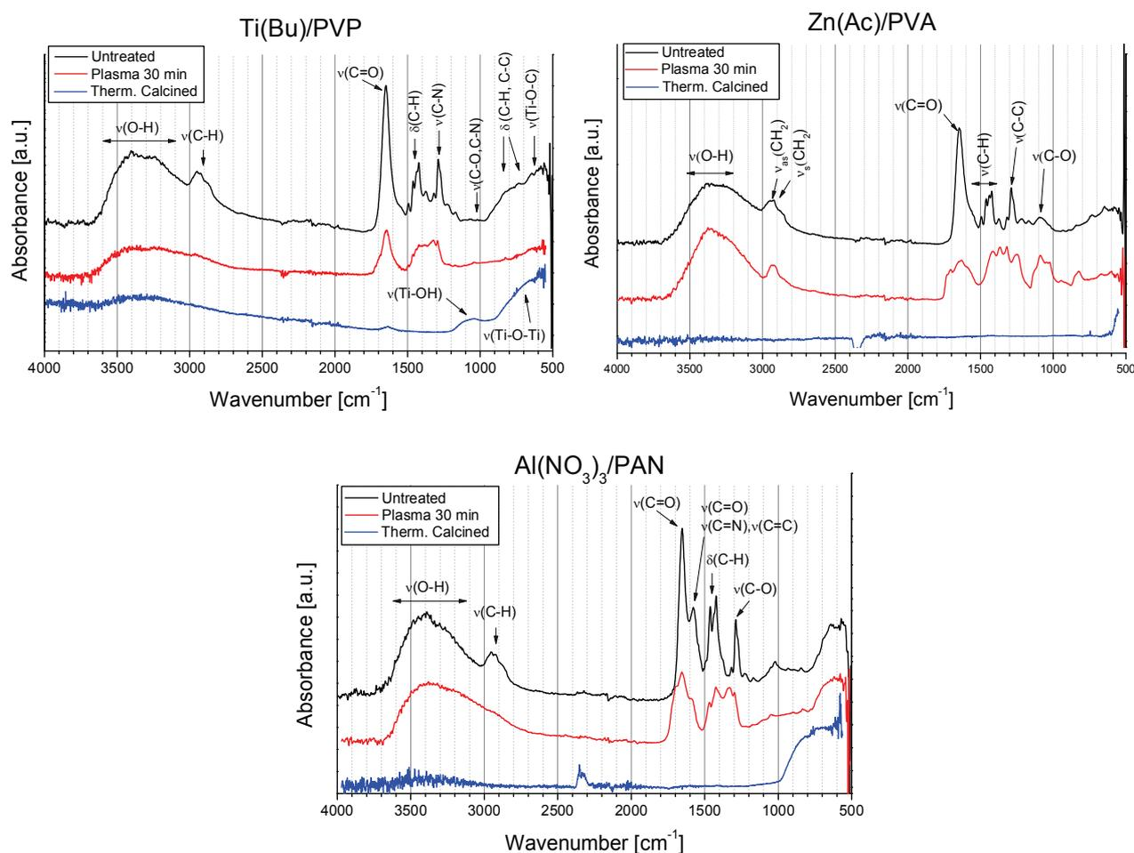
**Figure 2** ATR-FTIR spectra of hybrid nanofibers - untreated, treated by plasma for 30 minutes and thermally calcined inorganic fibers
