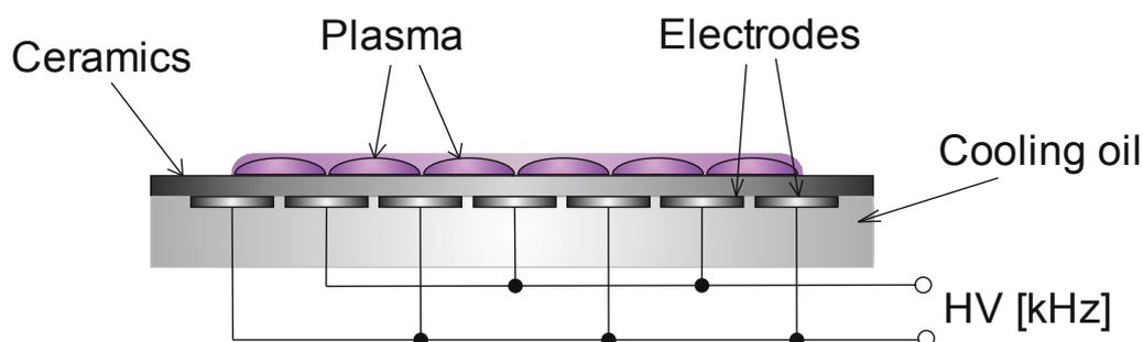
**Figure 1** Cross-section of DCSBD electrode system
