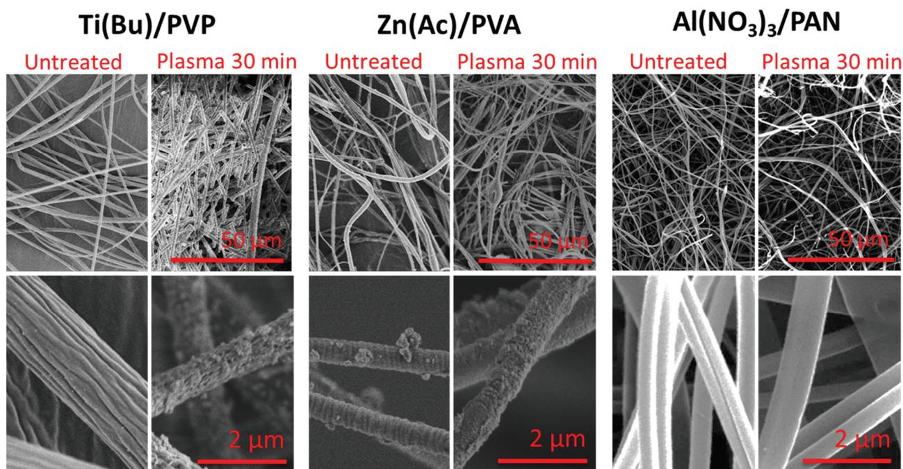
**Figure 4** SEM micrographs of precursor/polymer fibers before and after plasma treatment
