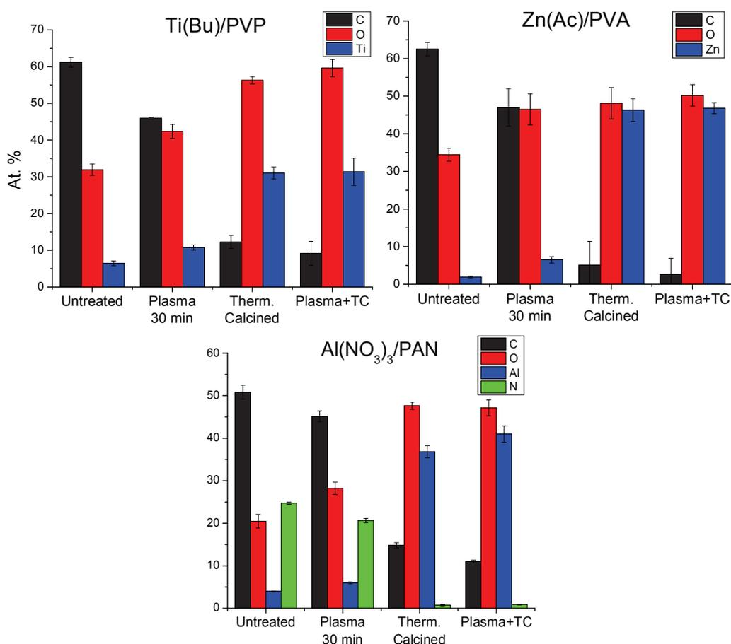
**Figure 3** Chemical compositions of hybrid nanofibers - untreated, treated by DCSBD plasma for 30 minutes and inorganic fibers prepared by conventional thermal calcination and combination of plasma pretreatment for 30 minutes and thermal treatment
