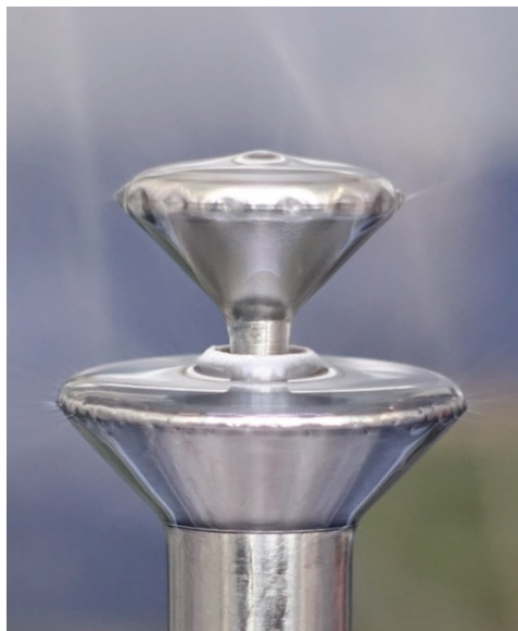
Figure 4 Detail view of the electrode heads under the AC-electrospinning process (upper head - PVAc solution, bottom head - PVB solution).
