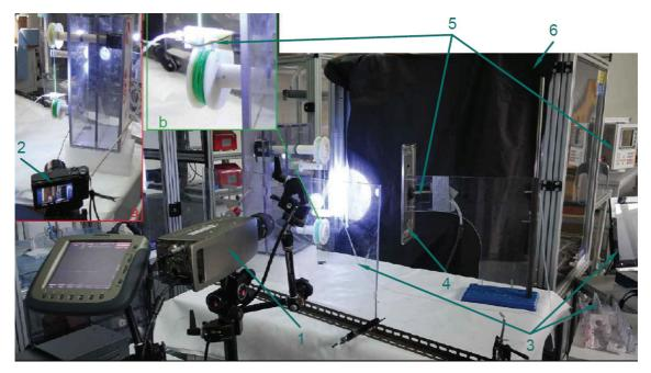
Figure 2 Measuring station for mobile string spinning electrode device
