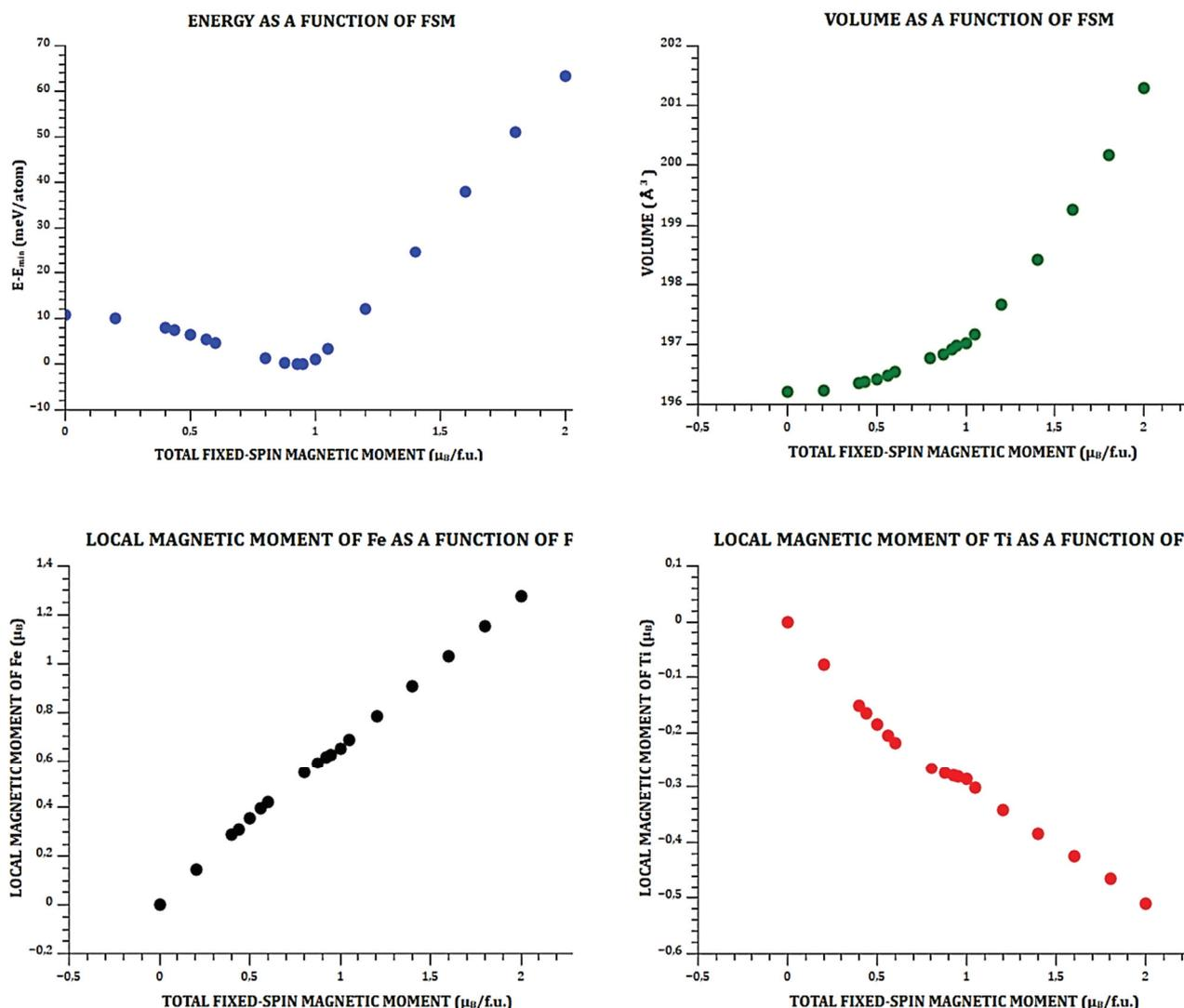
**Figure 2** Computed dependences of (a) the total energy (in eV/atom with respect to the lowest obtained energy), (b) a 16-atom supercell lattice parameter (in  $\text{\AA}$ ) and local magnetic moments of Fe (c) and Ti atoms (d) as functions of the fixed-spin value of the total magnetic moment per formula unit ( $\mu_B/f.u.$ ) of  $\text{Fe}_2\text{AlTi}$  with the  $L2_1$  structure
