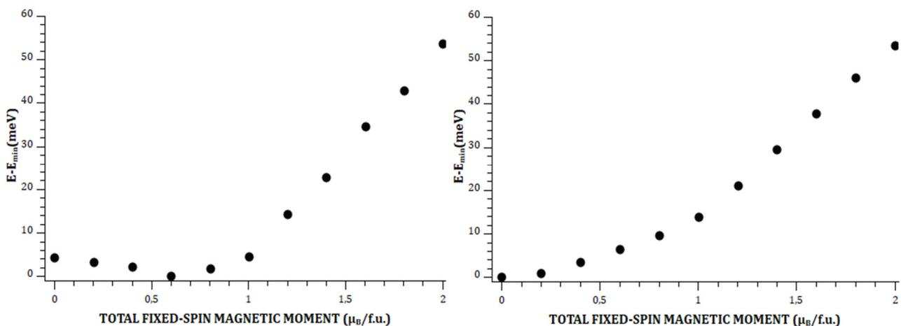
**Figure 3** Computed dependences of the total energy (in eV/atom with respect to the lowest obtained energy) for trigonal deformation with the strain of  $\varepsilon = 0.08$  (a) and  $\varepsilon = -0.08$  (b) as functions of the fixed-spin value of the total magnetic moment per formula unit ( $\mu_B$ /f.u.) of Fe<sub>2</sub>AlTi
