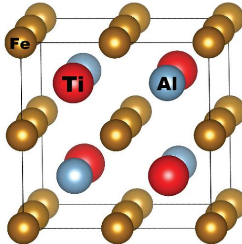
**Figure 1** Schematic visualization of a cube-shape 16-atom supercell of Fe<sub>2</sub>AlTi with four formula units used in our calculations
