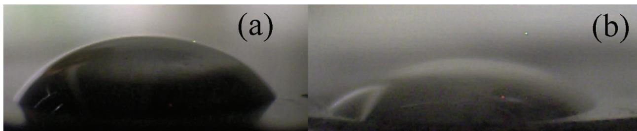
**Figure 3** Images from CCD camera of the silicone oil droplets on the GO (a) and GO- $\alpha$ -MeS (b) pellets
