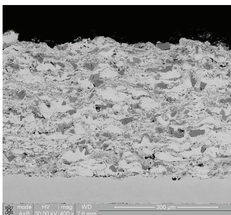
**Figure 2** SEM micrographs of cross-sections of the  $\text{Cr}_3\text{C}_2$ -25NiCr coating (back-scattered electron mode)
