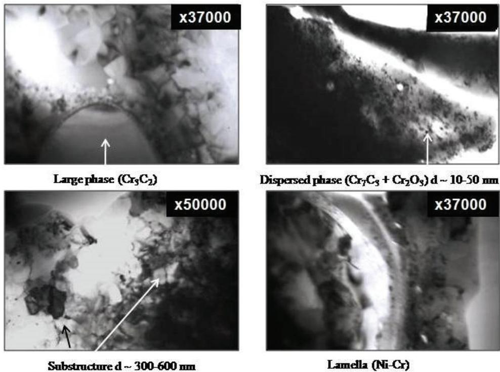
**Figure 5** The structure of the  $\text{Cr}_3\text{C}_2$ -25NiCr coating at a distance  $\sim 200\text{-}400 \mu\text{m}$  from the substrate
