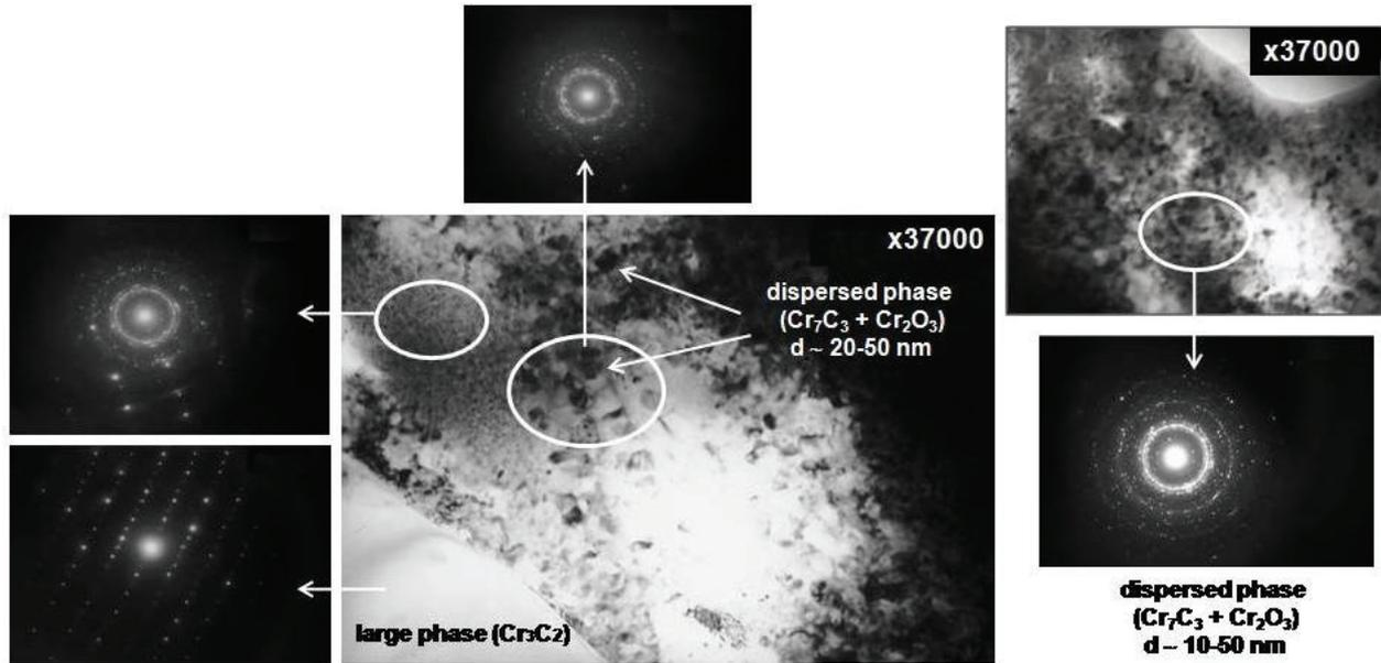
**Figure 4** The structure of the  $\text{Cr}_3\text{C}_2$ -25NiCr coating at a distance  $\sim 40 \mu\text{m}$  from the substrate
