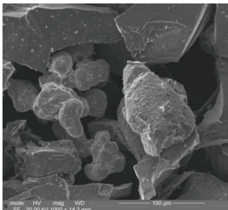
**Figure 1** SEM micrograph showing the morphology of the  $\text{Cr}_3\text{C}_2$ -25NiCr powder
