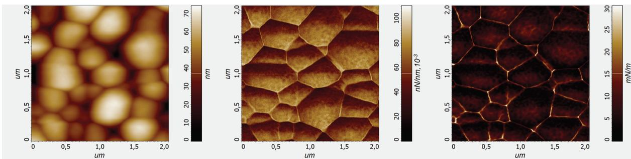
**Figure 5** Topography image (on the left), mapping of the stiffness (in the middle) and work of the adhesion map (on the right) for sample VI215
