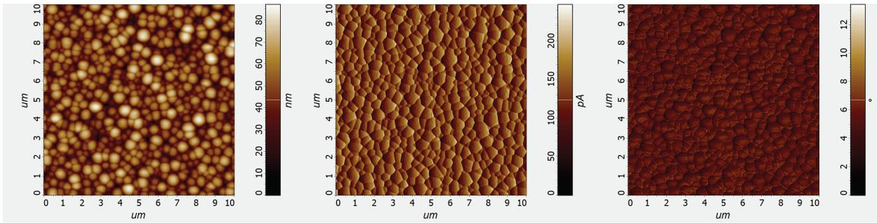
**Figure 4** Topography image (on the left), magnitude (in the middle) and phase (on the right) for sample VI215
