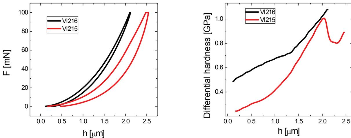
**Figure 3** Loading/unloading curves (on the left) and examples of differential hardness dependence on the indentation depth  $h$ . The differential hardness was calculated as the derivative of the load function with respect to the increasing contact area
