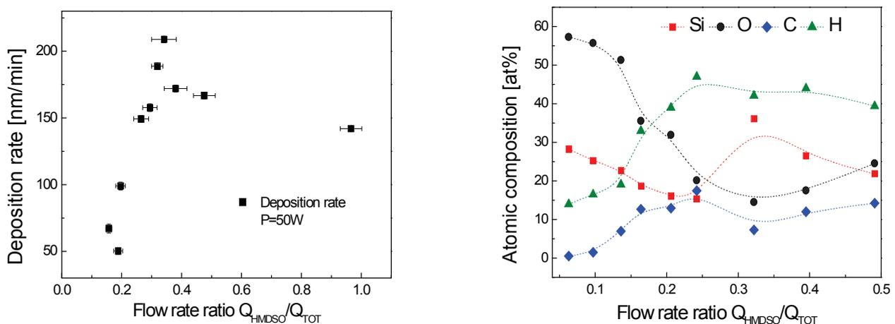
**Figure 1** Dependence of the deposition rate on the flow rate ratio for applied power of 50 W (on the left). Dependence of the film atomic composition on the flow rate ratio (on the right)
