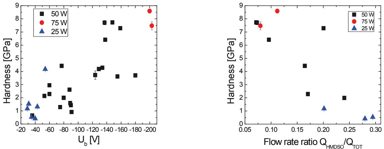
**Figure 2** Hardness dependence of prepared films on the DC bias voltage  $U_b$  (on the left) and hardness dependence on the flow rate ratio  $q$  (on the right) for three different applied powers of 25, 50 and 75 W
