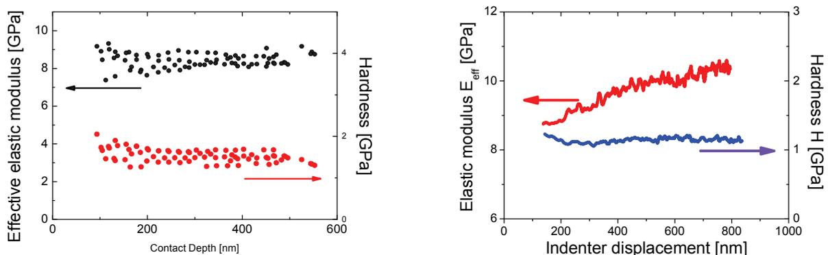
**Figure 6** Hardness and effective elastic modulus profiles obtained at several different places on the sample VI126 using quasistatic nanoindentation tests with 20 unloading segments (on the left) and nanodynamic analysis using oscillating load with frequency of 200Hz and load amplitude in the range from 1 to 10  $\mu$ N
