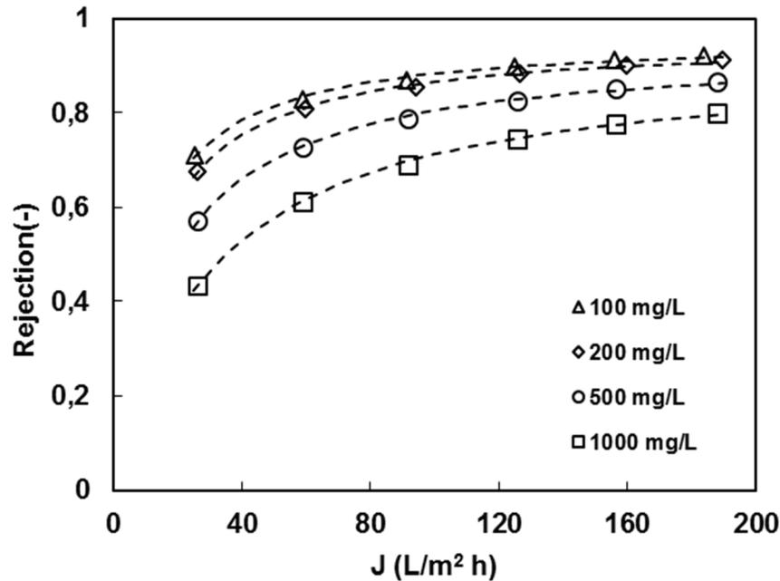
**Figure 2** Rejection of NaCl against flux (AFC 30 membrane). Experimental data (points) were fitted by Spiegler-Kedem model (dashed lines)
