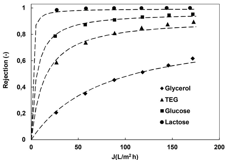
**Figure 1** Rejection of neutral solutes against flux (AFC 30 membrane). Experimental data (points) were fitted by the Spiegler- Kedem model (dashed lines)
