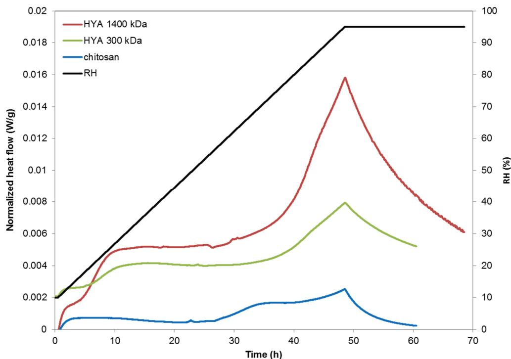
**Figure 4** The calorimetric responses to the adsorption of water vapor on chitosan and both hyaluronans in the RH perfusion cell. The heat flow data are connected with the left y-axis, the RH values for the black curve are displayed to the right y-axis
