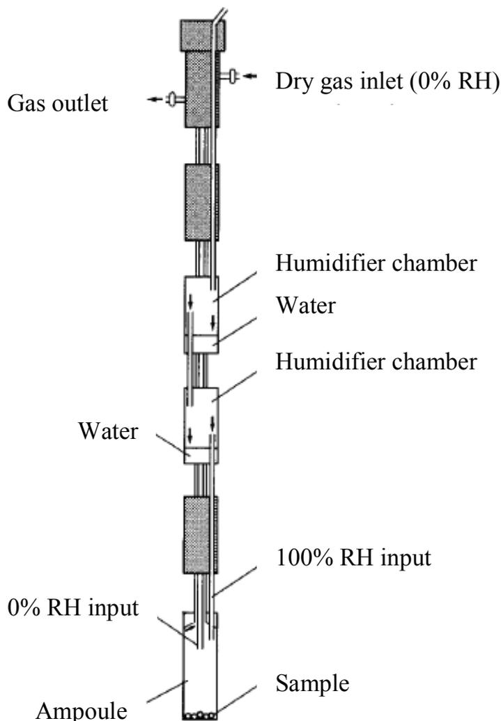
**Figure 1** A schematic of the RH perfusion cell [9]
