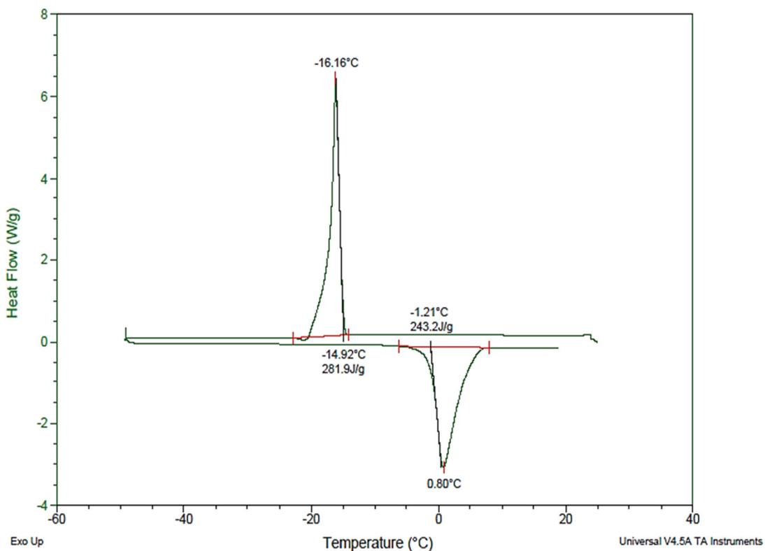
**Figure 2** DSC curves of chitosan measured after preparation
