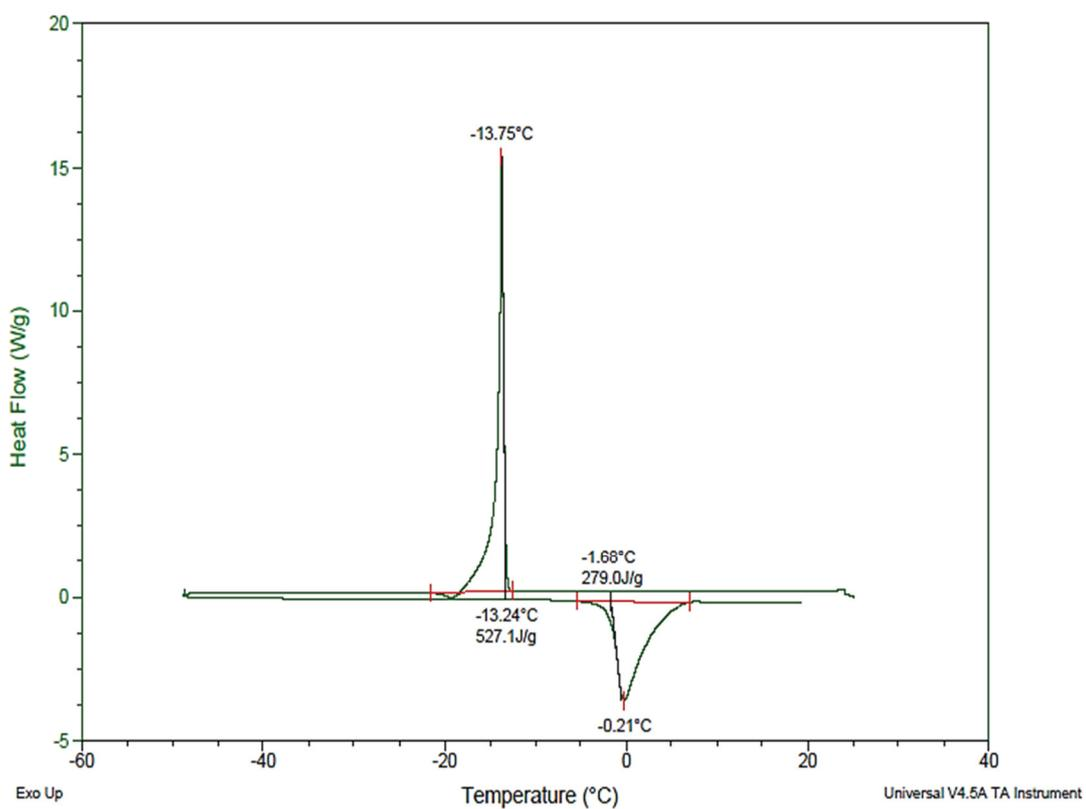
**Figure 3** DSC curves of chitosan measured within 24 hours of preparation
