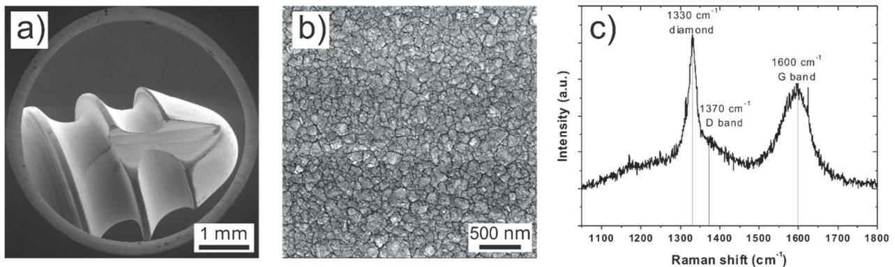
**Figure 1** SEM macroscopic and microscopic view of Ti screw together with typical Raman spectra
