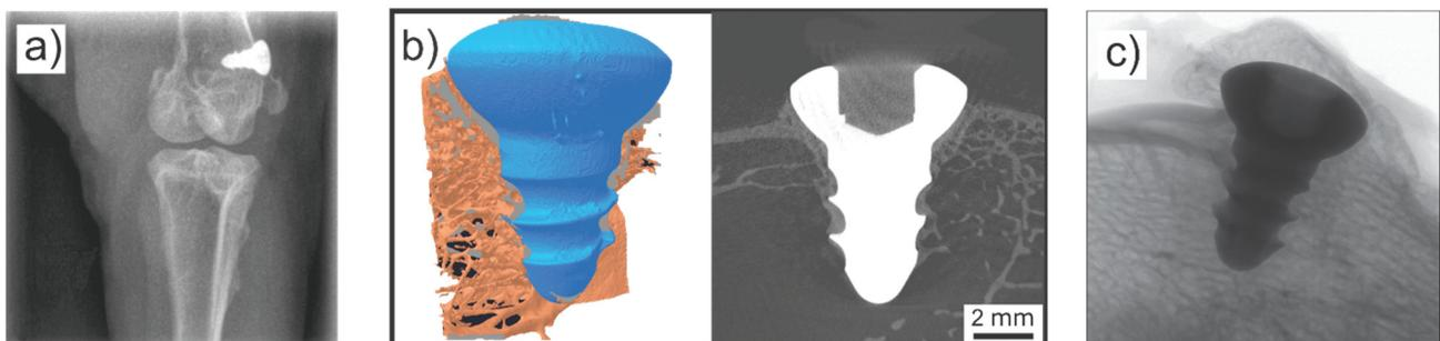
**Figure 2** X-ray image of implanted Ti screw (a), micro-CT image of reaction in the vicinity of Ti screw (b) and Ti screw with diamond over-coating layer six months after implantation
