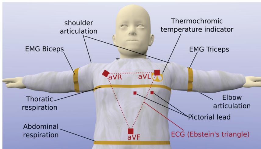
**Figure 2** Multiple sensing elements for continuous monitoring of physiological and movement data [7]
