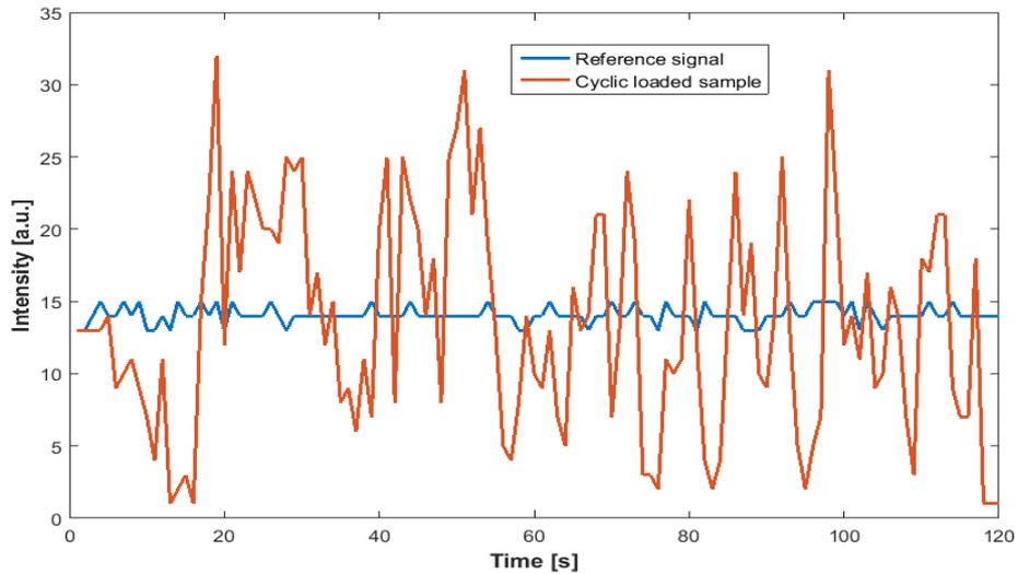
**Figure 4** Intensity of transmitted light signal in the reference (static) sample compared to the sample under dynamic loading
