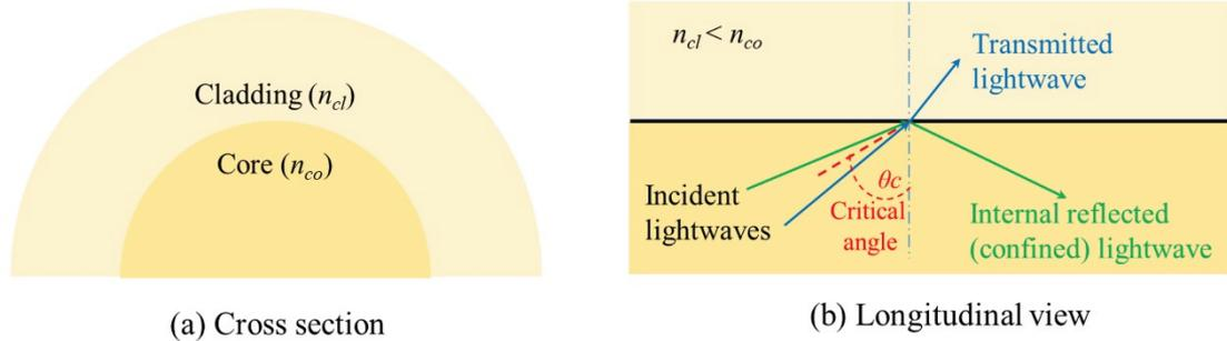
**Figure 1** The physical principle for lightwave confinement within the core of an optical fiber
