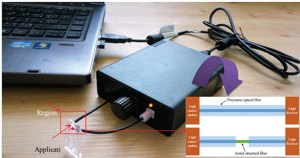
**Figure 3** Experimental setup. The inset schematically represents the arrangement for fiber testing
