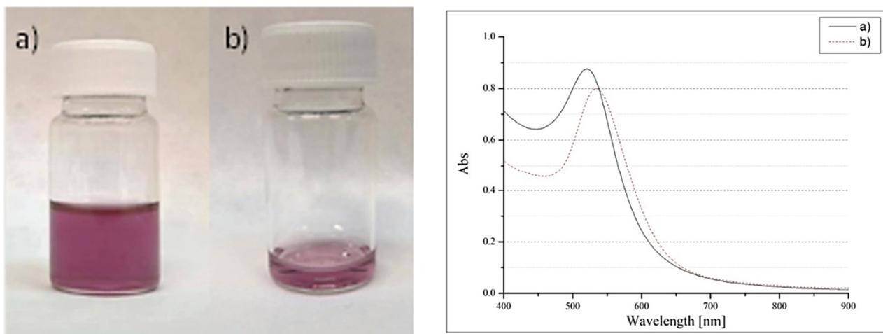
**Figure 1** On the left side: Digital images of nAu synthesized with: a) PHB-chit and b) PE. On the right side: Vis spectrum of nAu synthesized with: a) PHB-chit and b) PE
