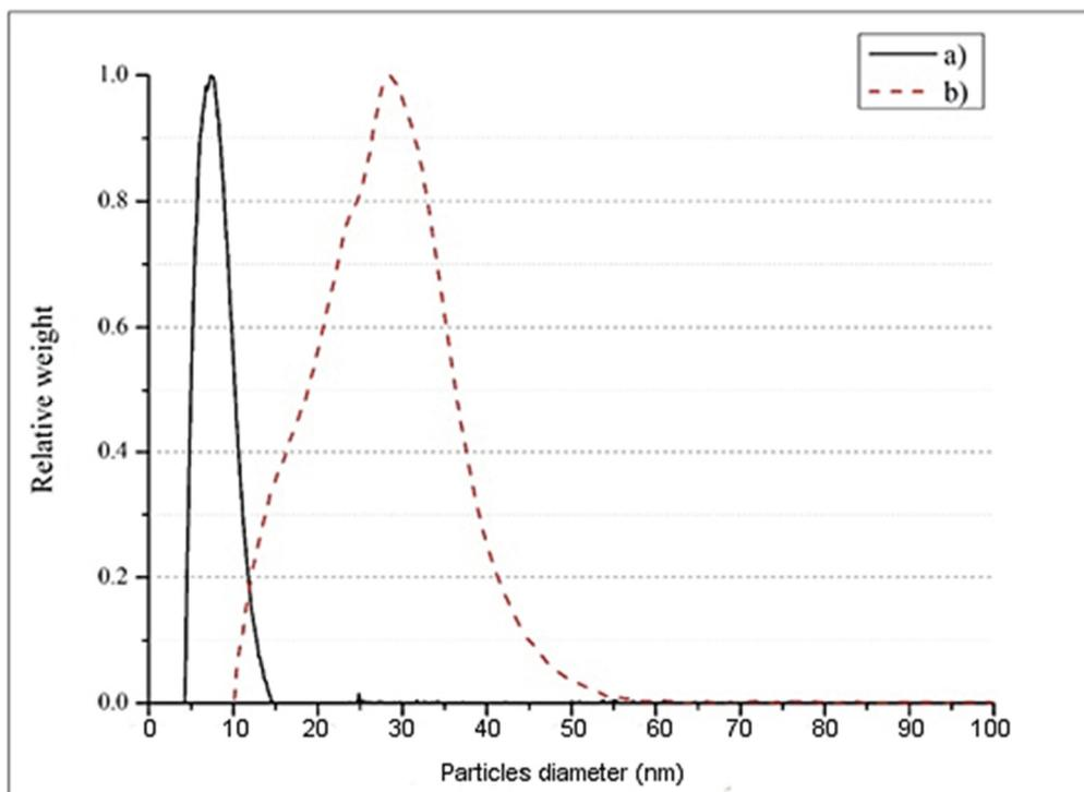
**Figure 2** The particle size distributions of nAu synthesized by: a) PHB-chit and b) PE
