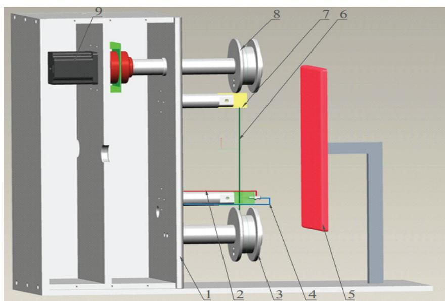
**Figure 1** Model of the mobile string spinning electrode device
