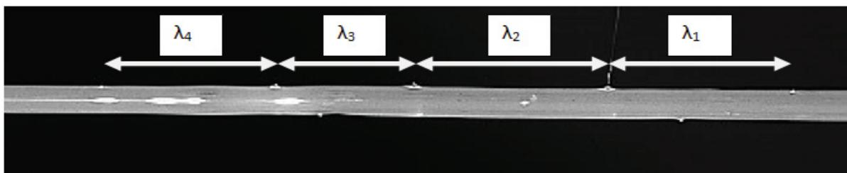
**Figure 3** Distance of Taylor cones, star cross-section, outer diameter 1.3 mm
