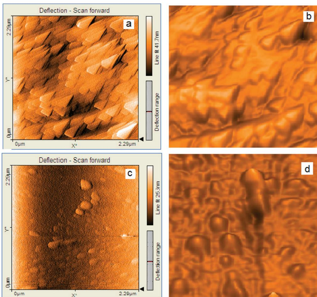
**Figure 5** 2D-AFM images for 2 micrometers of **Zn-PyPPP** treated with pyridine (a); and with 1-methylimidazole (c); 3D-AFM image in detail for **Zn-PyPPP** treated with pyridine (b); and with 1-methylimidazole (d)
