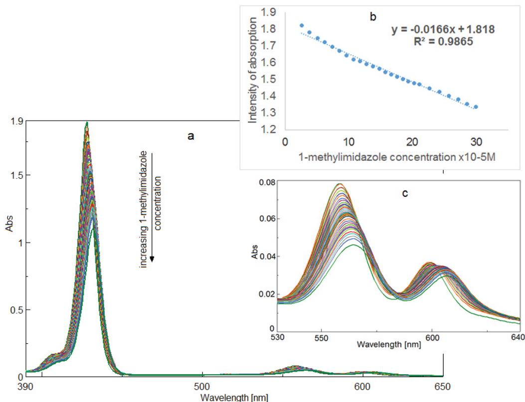
**Figure 4** Superposed UV-vis spectra for adding increasing concentrations of 1-methylimidazole to **Zn-PyPPP** solution in benzene (a); the linear dependence between the intensity of the Soret band and the 1-methylimidazole concentration (b); details of the Q bands (c)
