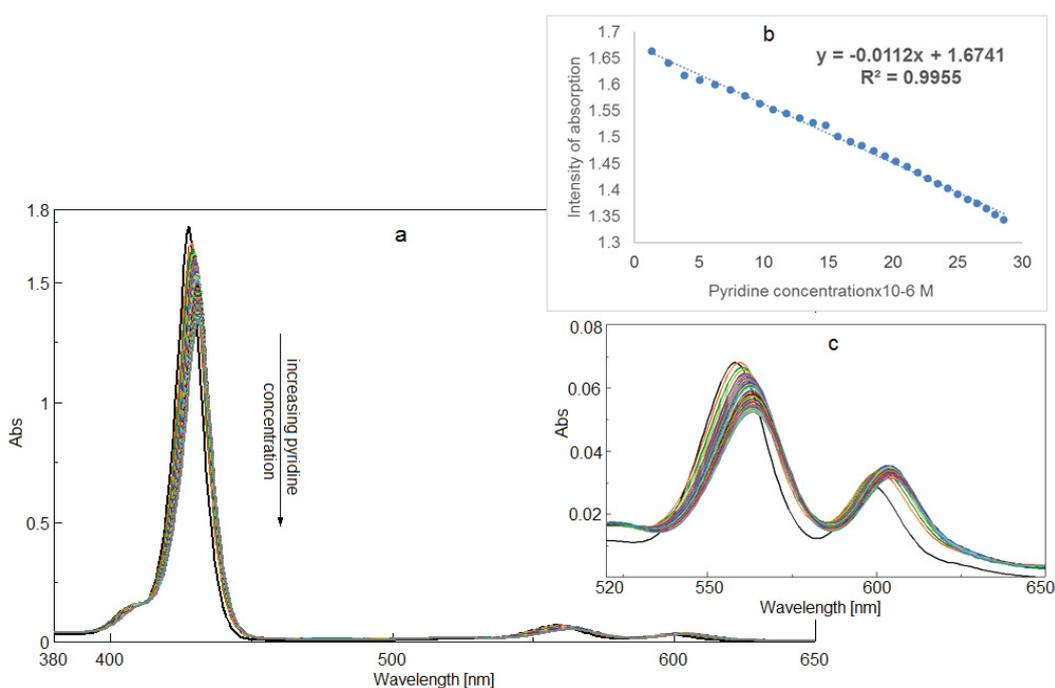
**Figure 3** The superposed UV-vis spectra for successive adding of pyridine solution to dilute **Zn-PyPPP** solution (a); the linear dependence between the intensity of the Soret band and the pyridine concentration (b); details of Q bands (c)
