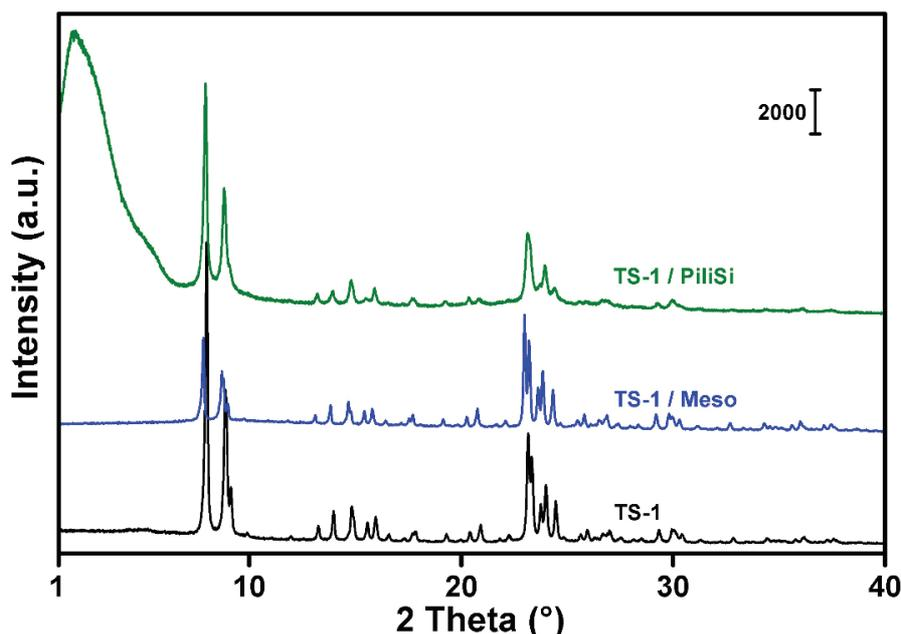
**Figure 1** X-ray powder diffraction patterns of calcinated Ti-catalysts. Conventional microporous titanositicate (TS-1), titanositicate with secondary prepared mesopores (TS-1 / Meso), top-down prepared layered titanositicate after Si-source pillaring (TS-1 / PiliSi)
