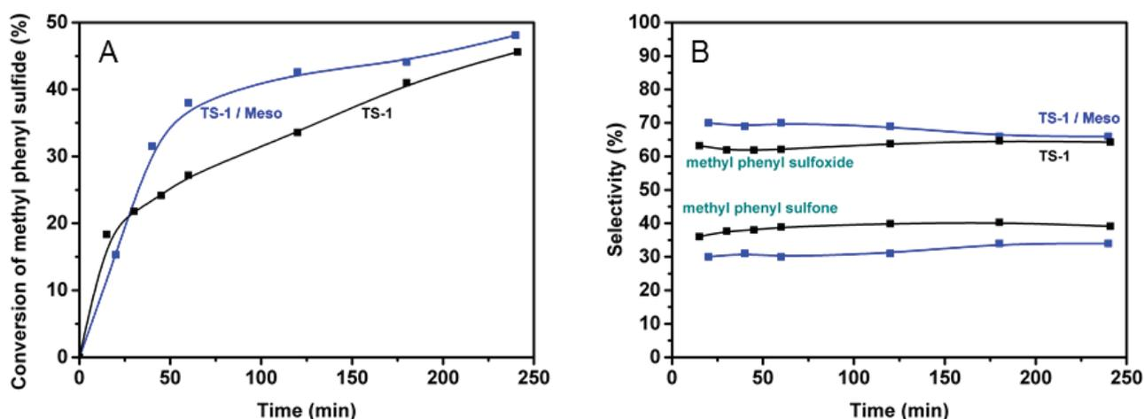
**Figure 3** Oxidation of methyl phenyl sulfide on microporous titanosilicate (TS-1) and titanosilicate with secondary prepared mesopores (TS-1 / Meso); conversion of methyl phenyl sulfide (A) and selectivity to the reaction products (B)
