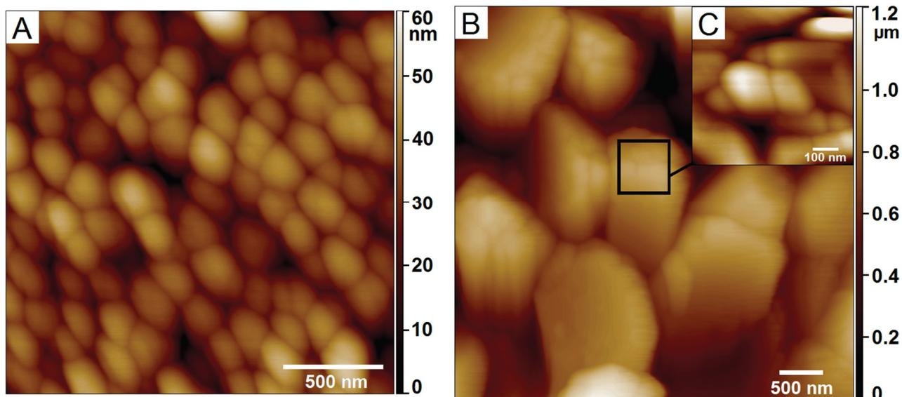
**Figure 2** AFM images of samples: microporous titanosilicate TS-1 (A), titanosilicate with secondary prepared mesopores TS-1 / Meso (B), and detailed view on surface of TS-1 / Meso grain showing mesopores (C)
