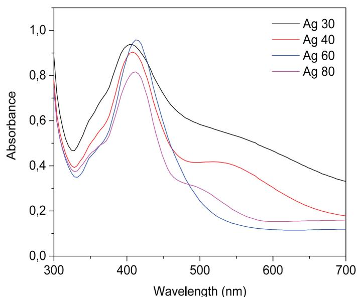
**Figure 2** Absorbance spectra of Ag NPs prepared under different temperatures; 30 °C, 40 °C, 60 °C, 80 °C
