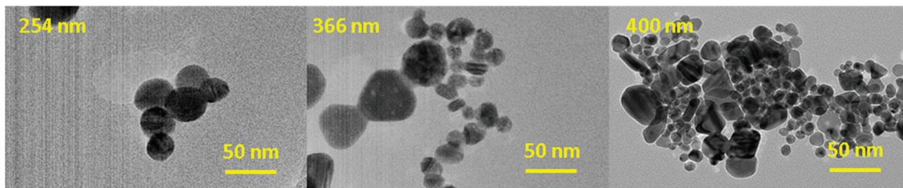
**Figure 4** TEM images of Ag NPs prepared under UV irradiation with three different wavelengths; 254 nm, 366 m, and 400 nm
