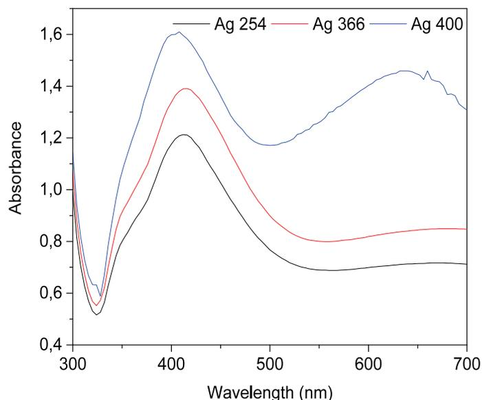
**Figure 5** Absorbance spectra of Ag NPs prepared under UV irradiation with three different wavelengths; 254 nm, 366 nm and 400 nm
