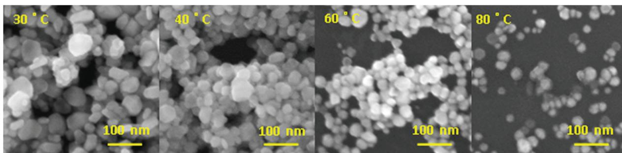
**Figure 1** SEM images of Ag NPs prepared at different temperatures: 30 °C, 40 °C, 60 °C, 80 °C
