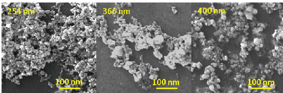
**Figure 3** SEM images of Ag NPs prepared under UV irradiation with three different wavelengths: 254 nm, 366 nm and 400 nm
