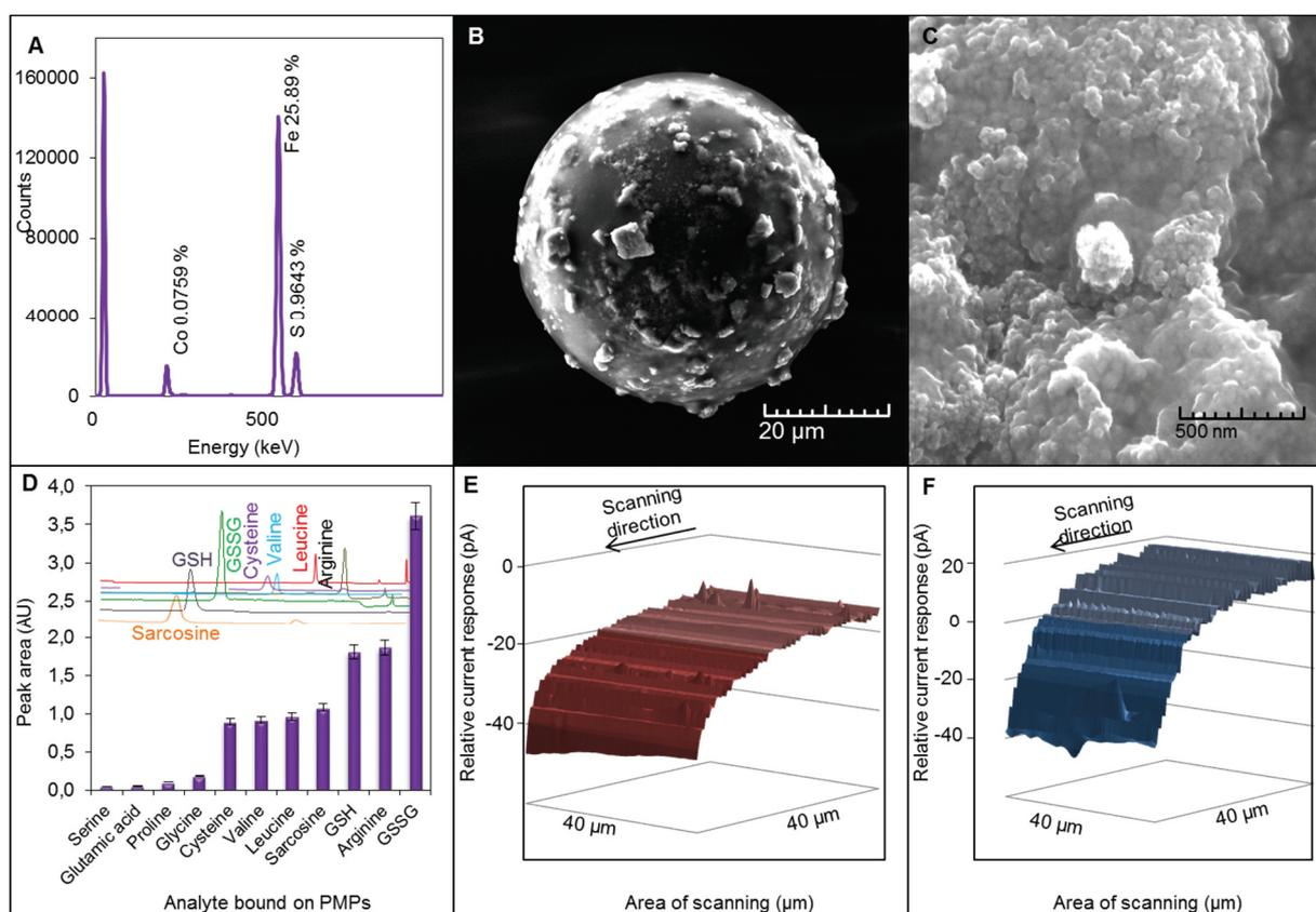
**Figure 2** Characterization of PMPs MAN16. **(A)** XRF showing elemental composition of MAN16. **(B)** SEM scan of MAN16 in resolution of 20  $\mu\text{m}$ . **(C)** SEM micrograph of MAN16 in resolution of 500 nm. **(D)** IEC results showing ability of MAN16 bound required substances specifically. **(E)** SECM scan showing relative current response without GSSG bound. **(F)** SECM scan with GSSG.
