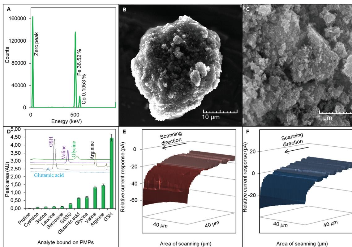
**Figure 1** Characterization of PMPs MAN3. **(A)** XRF showing elemental composition of paramagnetic microparticles. **(B)** SEM image in resolution of 10  $\mu\text{m}$ . **(C)** SEM scan in resolution of 1  $\mu\text{m}$ . **(D)** IEC results showing ability of MAN3 bound required substances specifically. **(E)** SECM scan showing relative current response of MAN3 without GSH bound. **(F)** SECM scan of MAN3 with GSH bound showing increased relative current response.
