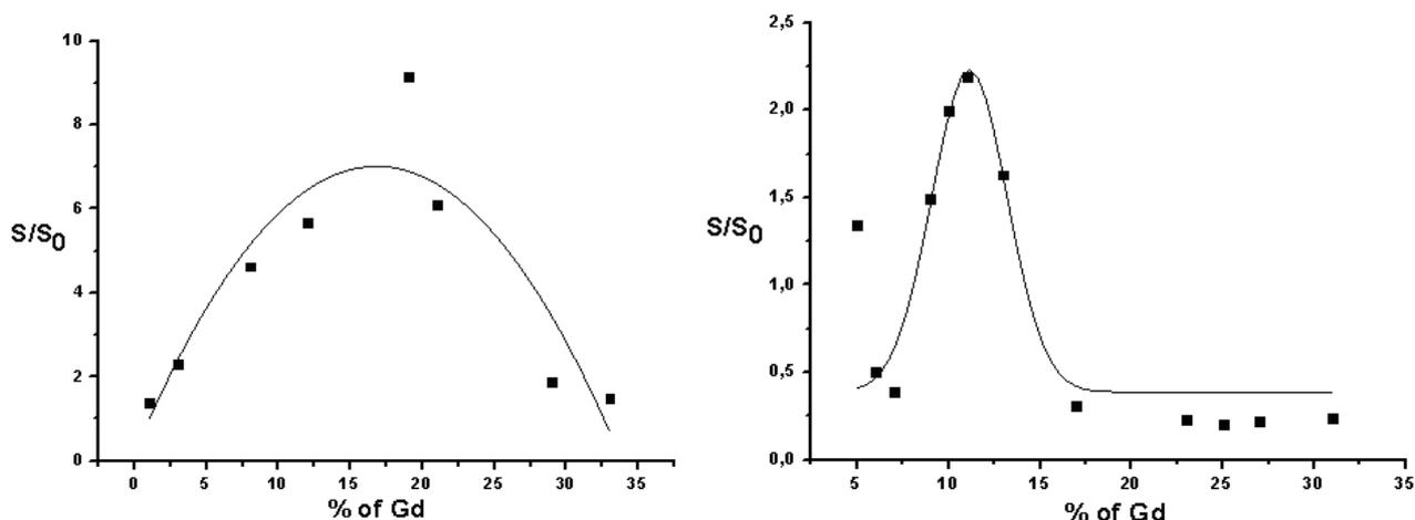
**Figure 3** Integral fluorescence area of Gd dope zinc oxide films. Gd concentration 1,3,8,12,19,21,29,33% (a) and 6,7,9,10,11,13,17,23,25,27,31 (b)
