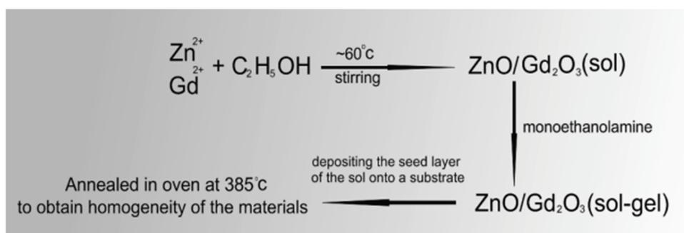
**Figure 1** The flow diagram for the preparation of the thin films modified ZnO
