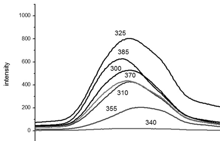
**Figure 2** Dependence of the fluorescence intensity of ZnO films on the annealing temperature after depositing the sol on a quartz substrate
