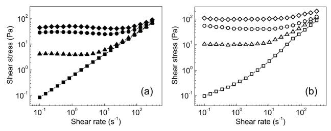
**Figure 2** Dependence of the shear stress,  $\tau$ , on the shear rate, g, for 5 wt. % silicone suspensions of aniline oligomers particles prepared in (a) neat GO and (b) GO- $\alpha$ -MeS, at various external electric field strengths, E, (kV.mm<sup>-1</sup>): 0 ( $\blacksquare$ , $\Box$ ), 0.5 ( $\blacktriangle$ , $\triangle$ ), 1.5 ( $\bigcirc$ , $\bigcirc$ ), 2.5( $\diamondsuit$ , $\diamondsuit$ )
