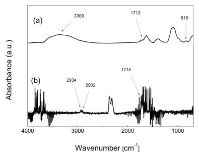
**Figure 1** FTIR spectra of the neat GO (a) and GO- $\alpha$ -MeS (b) particles
