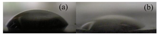
Figure 3 Images from CCD camera of the silicone oil droplets on the GO (a) and GO-a-MeS (b) pellets
