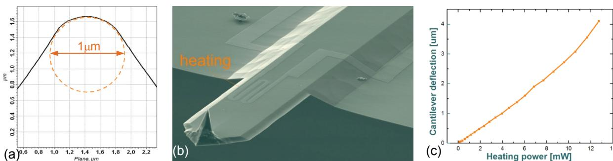
**Figure 5** (a) AFM profile of sharp edge of TGG1 calibration grating, which obtained using blunted tip with diameter of 1 μm (see left tip in Figure 4(b)). (b) AFM cantilever with meandered Al heater patterned by direct EBL and lift-off process. (c) Cantilever deflection as a function of electrical power used for the actuation.
