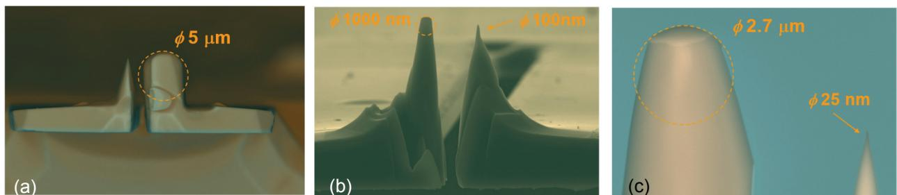
**Figure 4** Examples of final probes. Sharp tips with a sub-100 nm curvature diameter can be prepared by a sharpening process. Blunting process allows setting the tip curvature diameter in a range of 100 nm - 5000 nm. (Images were colorized in post-processing).
