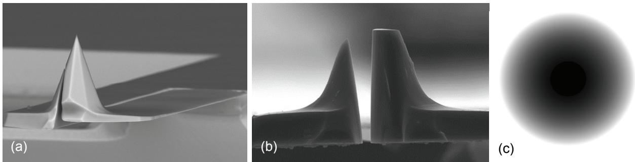
**Figure 3** (a) Commercial AFM probe after splitting by FIB, (b) tip apex has to be cut prior to forming into spherical shape, (c) mask pattern used for forming a sphere at the large tip
