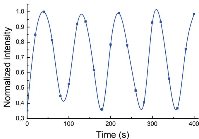
**Figure 4** The time evolution of the maximal intensity of the Ar (707 nm) spectral line
