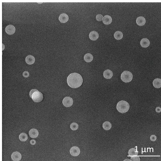
**Figure 5** SEM image of hydrocarbon nanoparticles produced by GAS
