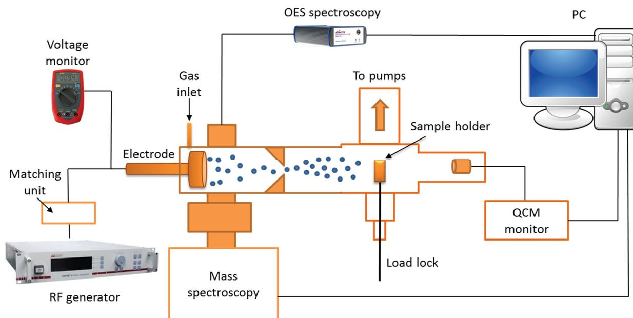
**Figure 1** Simplified scheme of the experimental set-up
