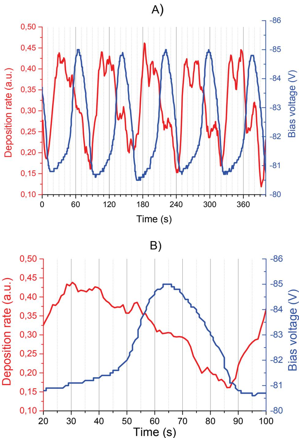
**Figure 2** Time evolution of the nanoparticle deposition rate and the bias voltage during the GAS operation (A) and details of one cycle with snapshots made every 5 s (B)
