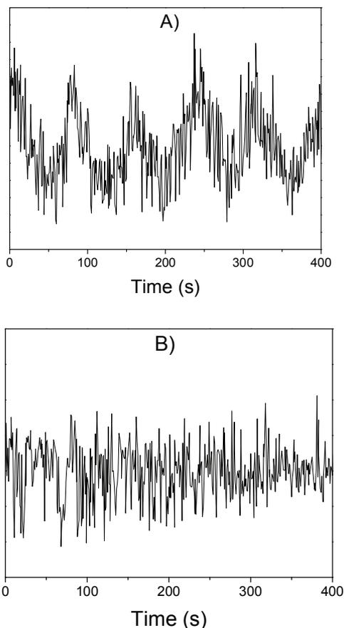
**Figure 3** Time dependences of the selected peaks in the mass spectra: a) for mass 86 ( $C_6H_{14}$  precursor); b) for mass 36 (Ar)
