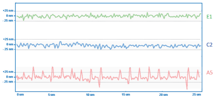
Figure 5 Comparison of the smoothing algorithms results: AFM scan along the grating line
