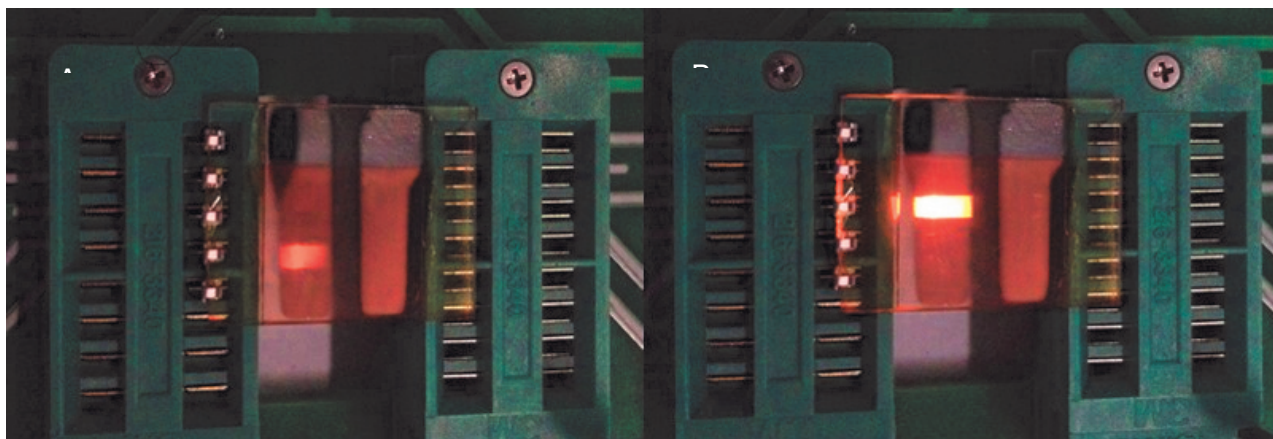
Figure 5 Prepared PLED devices: A - neat MEH-PPV as an active layer, B - MEH-PPV/ZnO 12.5 wt. % as an active layer, operated at 10 V
