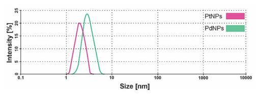
Figure 2 Characterization of aqueous solutions with platinum and palladium nanoparticles by dynamic light scattering
