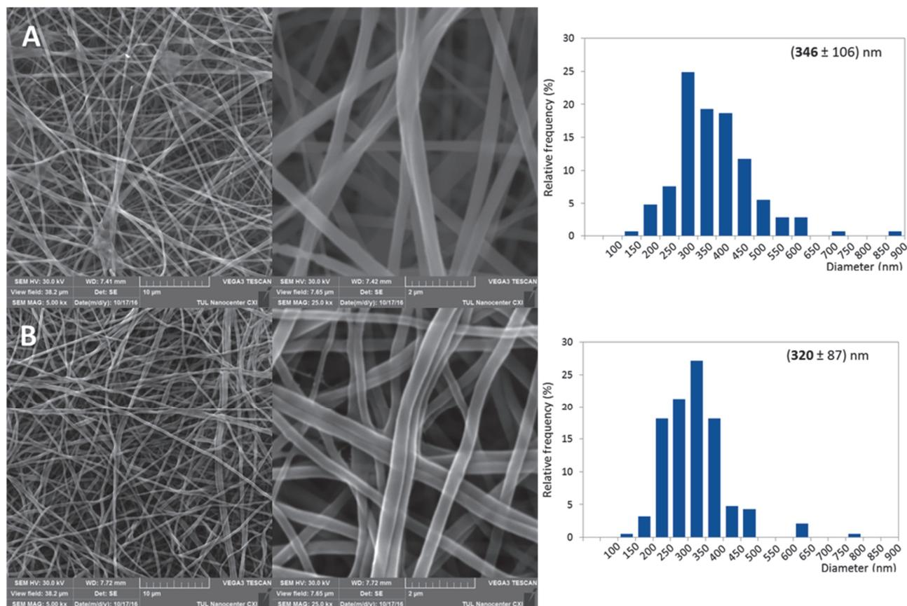
**Figure 1** Morphology of SF nanofibres (A) prior the stabilization and (B) after the stabilization. SEM under magnification 5.000 and 25.000 (bar1 = 10  $\mu\text{m}$ , bar2 = 2  $\mu\text{m}$ ), histogram of relative frequency of the fiber diameters, mean  $\pm$  S.D. (n=100)
