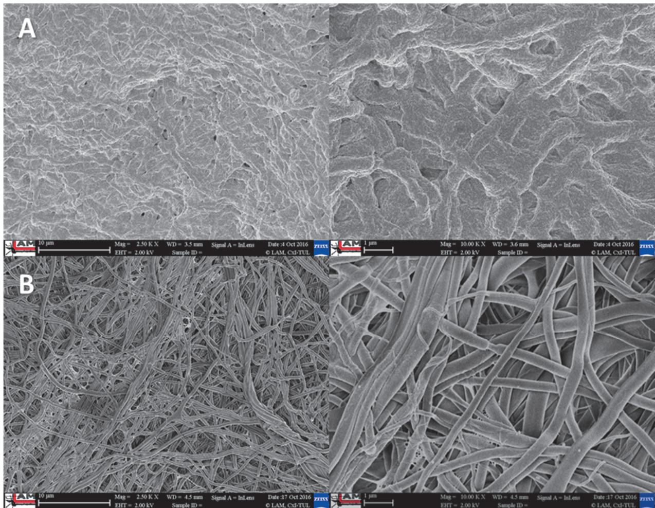
**Figure 2** Morphological changes observed after 72 hours of degradation in vitro in SBF. (A) Unstabilized and (B) stabilized Silk fibroin nanofibres. SEM under mag. 2.500 and 10.000 (bar1 = 10 µm, bar2 = 1 µm)
