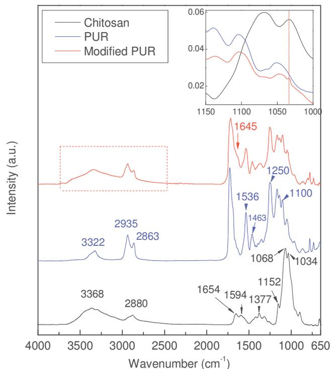
**Figure 3** Infrared spectra of neat chitosan, polyurethane foil and polyurethane foil grafted with chitosan
