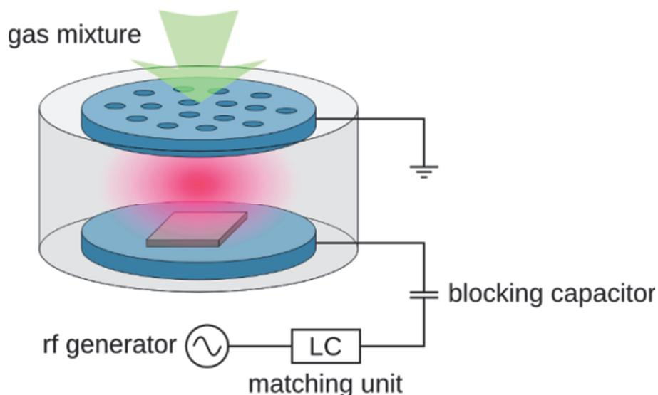
**Figure 1** Schematic drawing of the plasma set-up<sup>[8]</sup>
