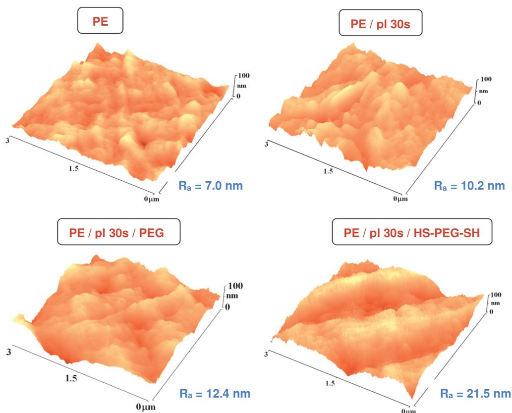
**Figure 1** AFM images and the surface roughness of pristine PE, PE treated by plasma for 30 s and grafted by PEG and HS-PEG-SH
