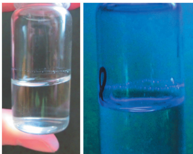
Figure 3 The condensed phase on the wall of the vial. Left - natural light, right - UV
