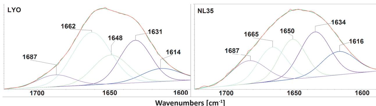
**Figure 6** Comparison of the deconvoluted ATR-FTIR spectra of lyophilized collagen (LYO) and the NL35 material
