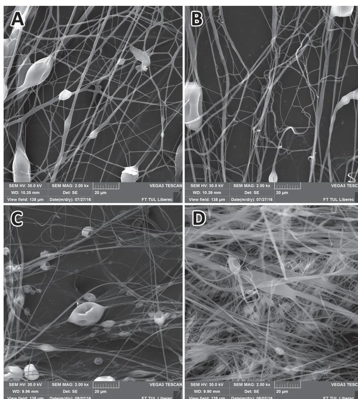
**Figure 3** Representative SEM images of samples prepared employing the needleless (A, B) and needle (C, D) centrifugal force spinning of the collagen solutions (with PEO) with a concentration of 12 wt% and circumferential velocities of 15 m.s<sup>-1</sup> (A, C) and 35 m.s<sup>-1</sup> (B, D) (mag. 2,000x)
