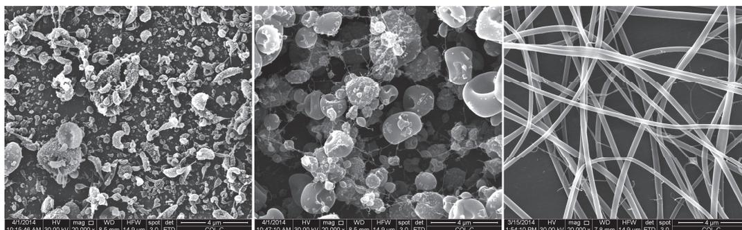
**Figure 1** Representative SEM images of samples electrospun from collagen solutions (without PEO) with concentrations of (from left) 4, 8 and 16 wt% (mag. 20,000x)
