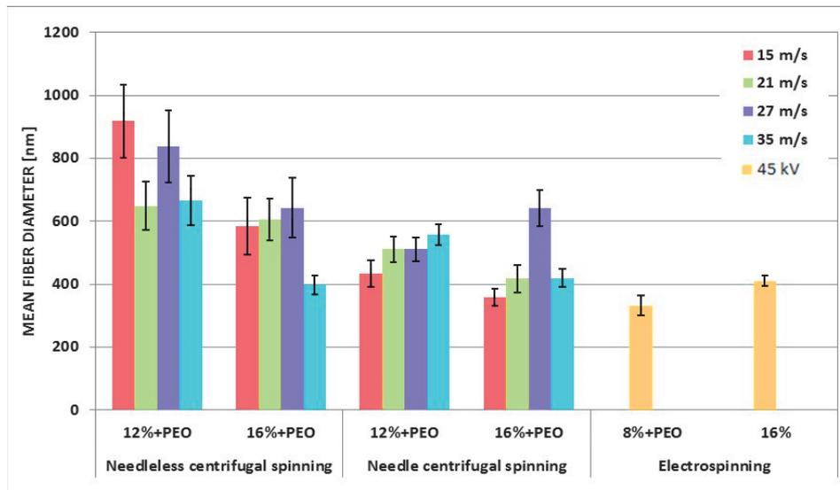
**Figure 4** Graph illustrating the effect of solution concentration and the applied technology on the diameter of the fibers
