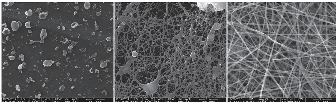
**Figure 2** Representative SEM images of samples electrospun from collagen solutions (with PEO) with concentrations of (from left) 4, 6 and 8 wt% (mag. 10,000x)
