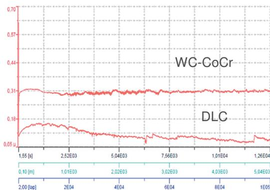
**Figure 7** Friction coefficient of WC-CoCr and DLC coating
