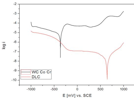
**Figure 6** Tafel plots for WC-CoCr and DLC in 3.5% NaCl solution
