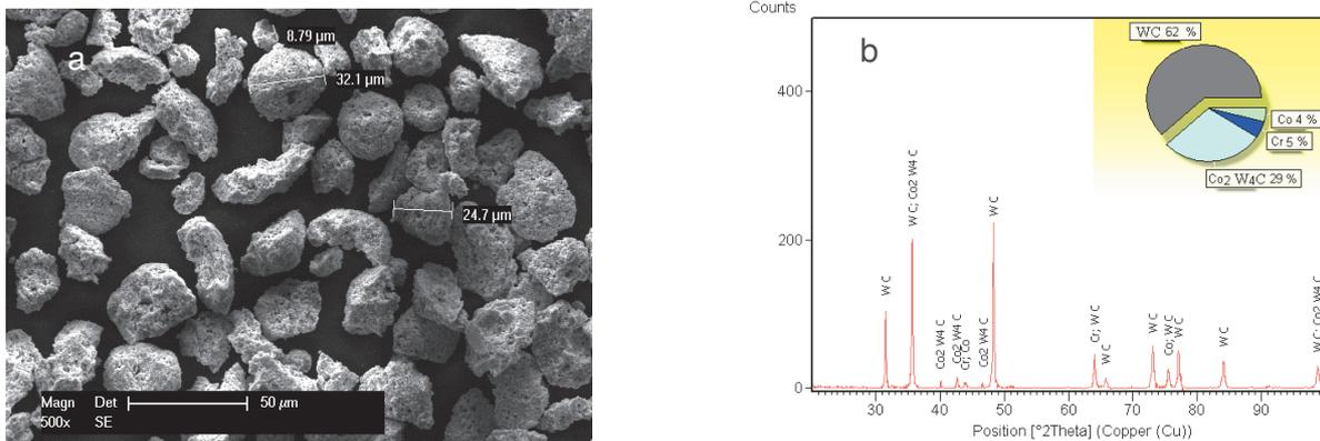
**Figure 1** SE micrograph of the WC-CoCr powder (a) and its X-ray diffraction pattern (b)
