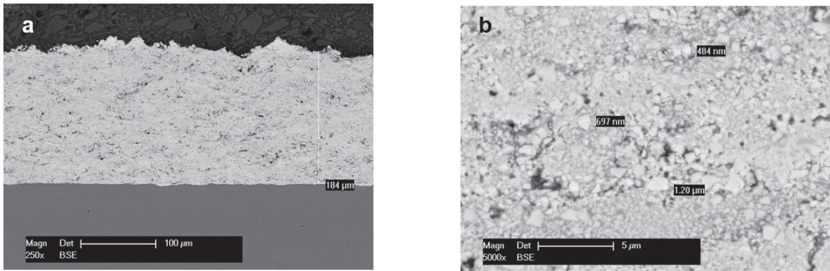
**Figure 2** SEM micrographs of the as sprayed WC-CoCr coating as (a) overview and (b) size of the WC particles
