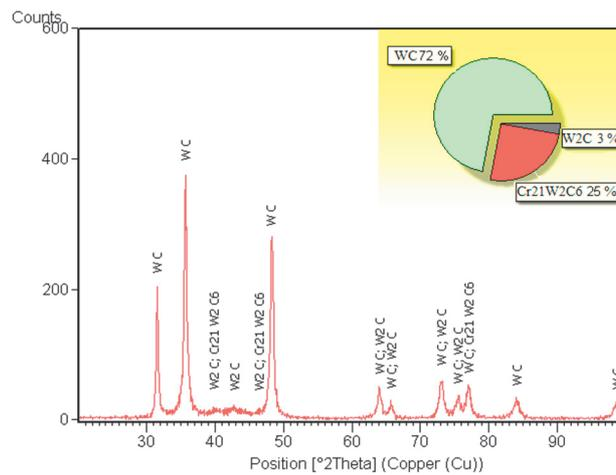
**Figure 3** X-ray diffraction pattern of the WC-CoCr coating
