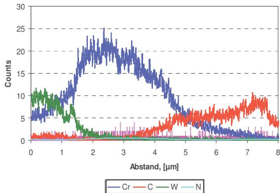
**Figure 5** EDX line-scan of the DLC/WC-CoCr multi-layered coating
