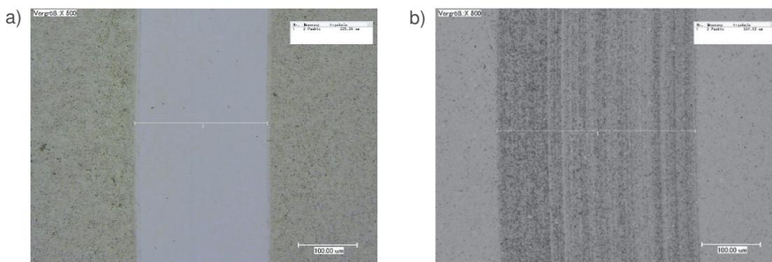
**Figure 8** Wear track of the (a) WC-CoCr and the (b) DLC coating respectively
