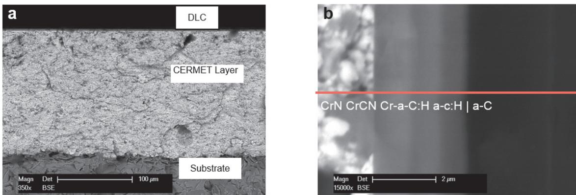
**Figure 4** SEM micrographs of the cross-sectioned DLC/WC-CoCr coatings systems as (a) overview and of the (b) EDX line scan
