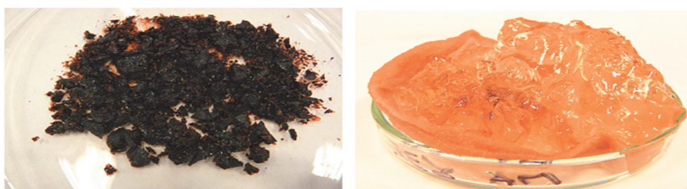
Figure 1 a) Xerogel of superabsorbent polymer b) Swollen superabsorbent polymer
