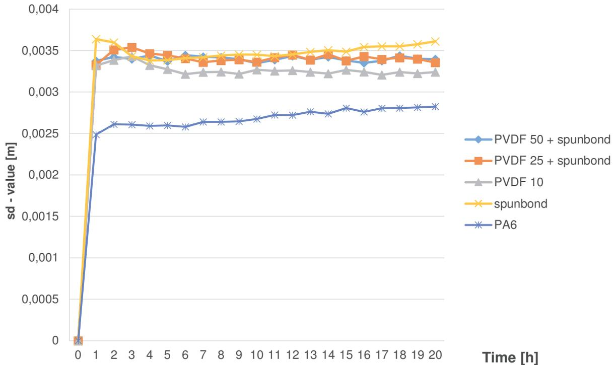
**Figure 5** Water vapour diffusion equivalent air layer thickness  $s_d$  of PVDF nanotextiles and PA6 nanotextile calculated from the diffusion measurement as a function of time
