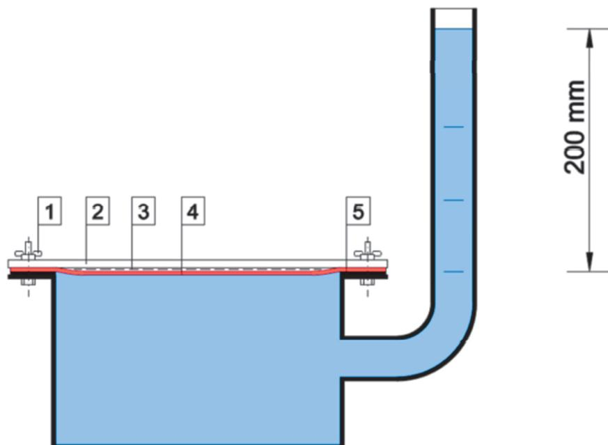
**Figure 3** The schema of experimental device for measuring watertightness by the method of constant loading by a water column of 200 mm (1 - Sample holding device, 2 - Plexiglass, 3 - Laboratory filter paper indicates watertightness, 4 - Sample, 5 - Rubber ring)
