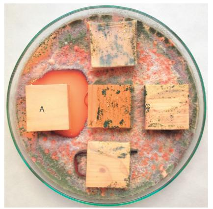
Figure 2 Plate with wooden samples at 11th day of experiment
