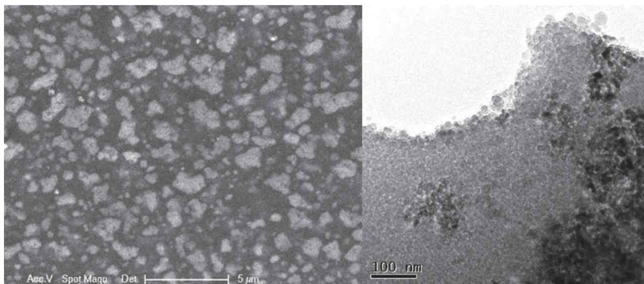
**Figure 2** SEM (left) and TEM (right) micrograph of TiO<sub>2</sub>-SiO<sub>2</sub> nanocomposite
