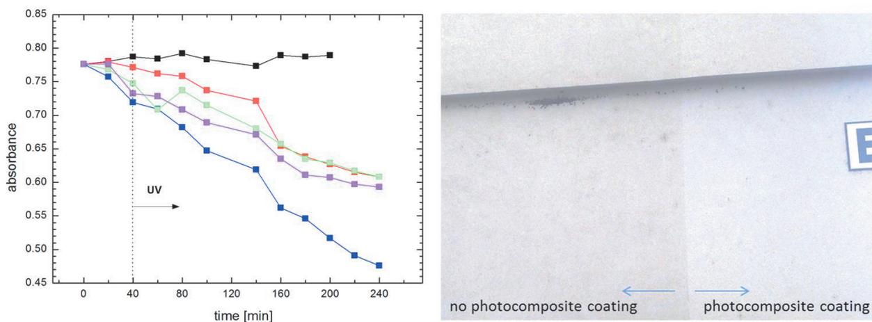
**Figure 4** The course of photocatalytic degradation of methylene blue on TiO<sub>2</sub>-SiO<sub>2</sub> nanocomposite coatings on **acrylic paint**, **silicone paint**, **lime plaster**, and **silicate paint** (left graph, **black** curve relates to blank experiment); photography of building facade comparing appearance of coated and non-coated places after 2 years of out-door exposition (right)
