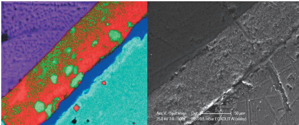
**Figure 3** EDS mapping (left) and SEM micrograph (right) of cross-section of TiO<sub>2</sub>-SiO<sub>2</sub> nanocomposite coating
