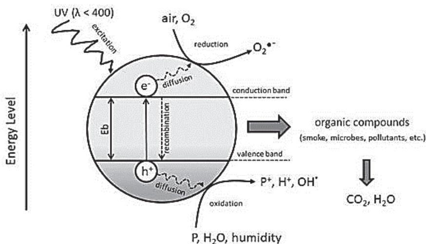
**Figure 1** Illustration of photocatalytic processes occurring on semiconductor particle upon irradiation
