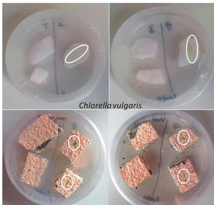
**Figure 5** The algae growth testing on white marble (up) and on plaster (down). The samples on the right (left) part of petri dishes are not coated (coated) with TiO<sub>2</sub>-SiO<sub>2</sub> nanocomposite. The algae are marked by a white circle
