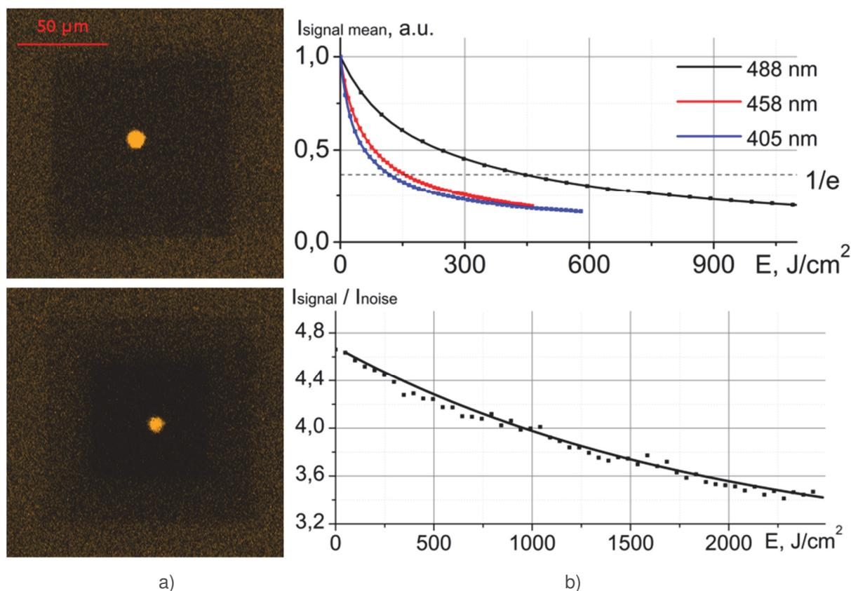
**Figure 4** Images of bleached area (notice darker squares around the bright marked in the center) in Chromone: PMMA sample and corresponding dependencies of luminescence signal and signal/noise(background) ratio on exposure values
