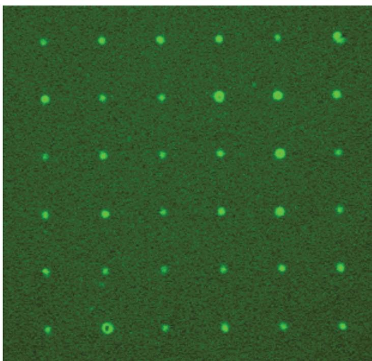
**Figure 3** Rectangular grid pattern of multiphoton-recorded fluorescent marks in Chromone:PMMA sample
