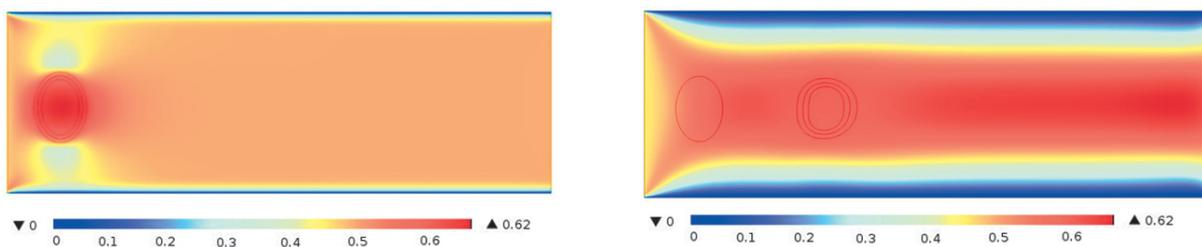
**Figure 7** Movement of the drop in the created flux [m/s]. The red path of the right picture is representing stream with highest velocity of the supposed particle transport
