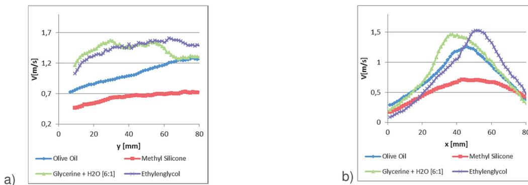
**Figure 2** Profile plots of the moving droplets taken a) vertical line, b) horizontal line showing less electric interaction between Methyl Silicone and induced HV field
