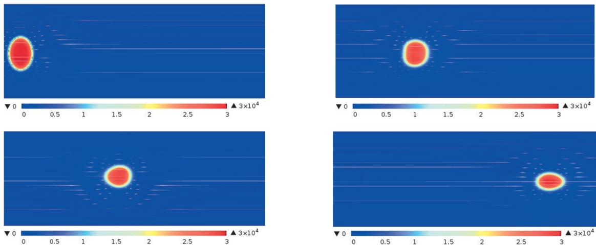
**Figure 6** Movement and deformation of the drop in electric field powered by 30 kV. Red color representing high intensity of the field in the droplet
