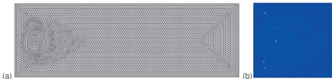
**Figure 4** Tetragonal mesh (a) followed with detailed picture (b) of the vicinity of the drop
