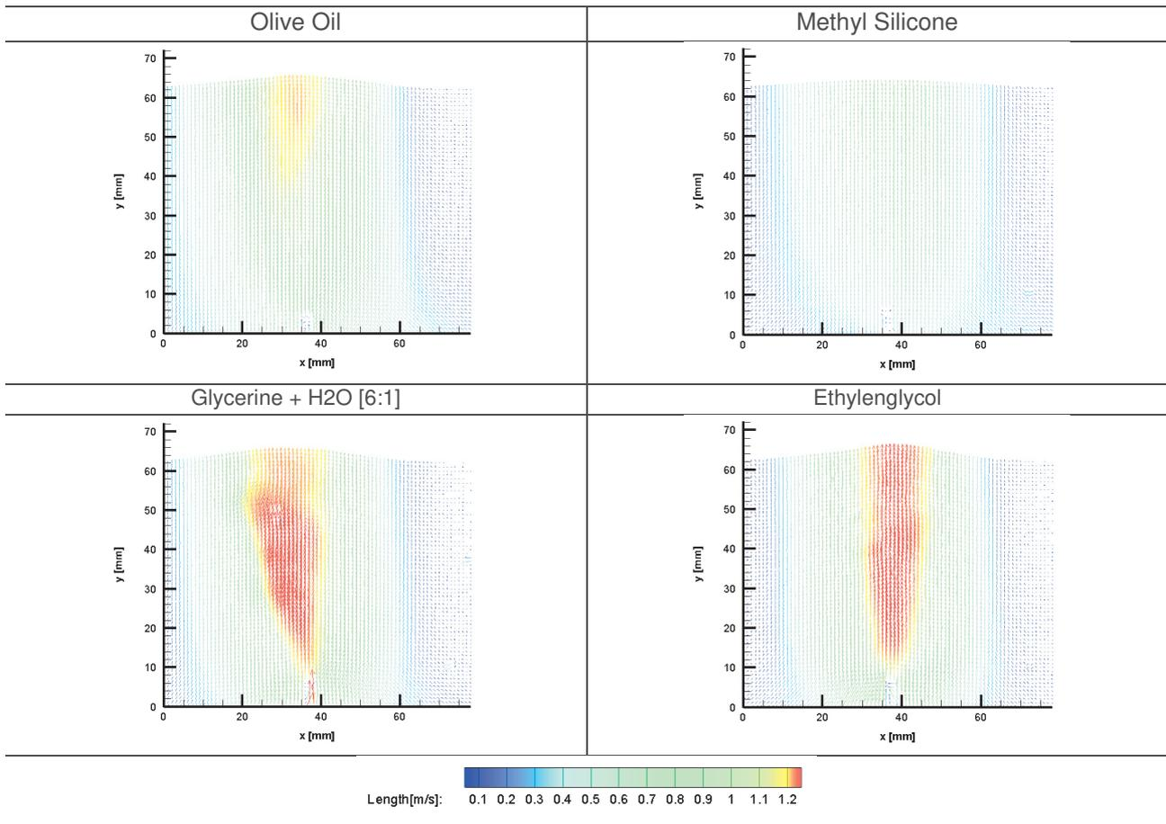
**Figure 1** Vector maps of monodisperse droplet movement induced by electric field. Different particles are moving by different velocities. Mixture of Glycerine with water and Ethylenglycol are reacting more with HV field therefore generating higher speeds (red vectors)
