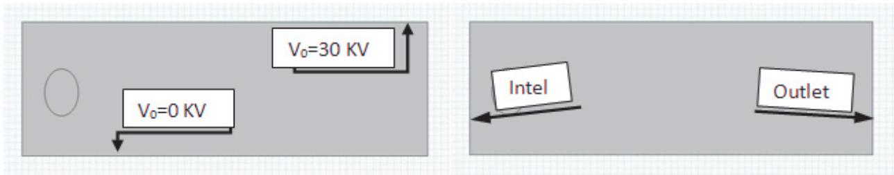
**Figure 5** Boundary conditions for the input and output of electrical potential and flux ranging from zero voltage to 30 kV
